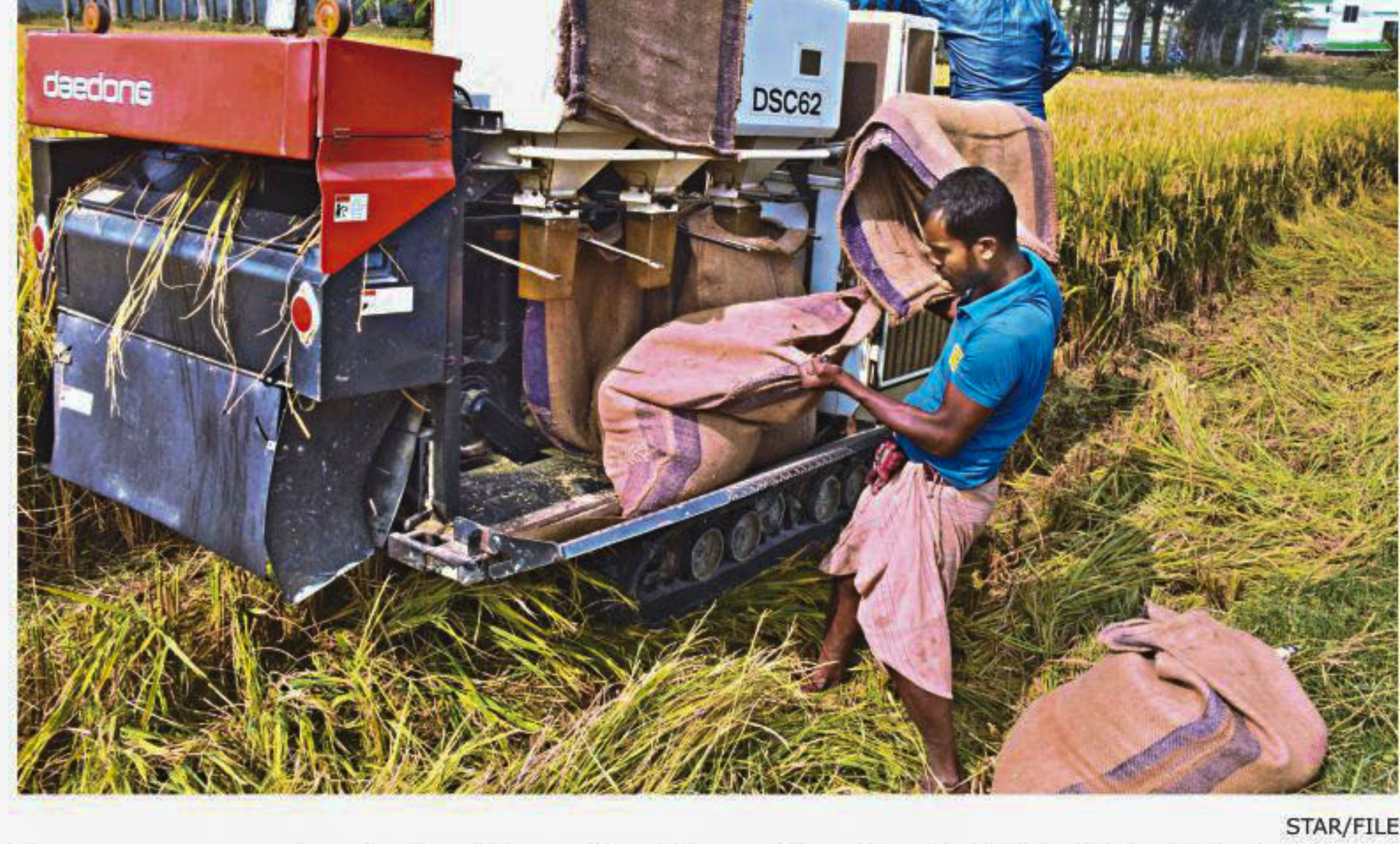
Farmers use a machine for threshing and packing paddy, all on the field, at Lakutia in Barishal.
