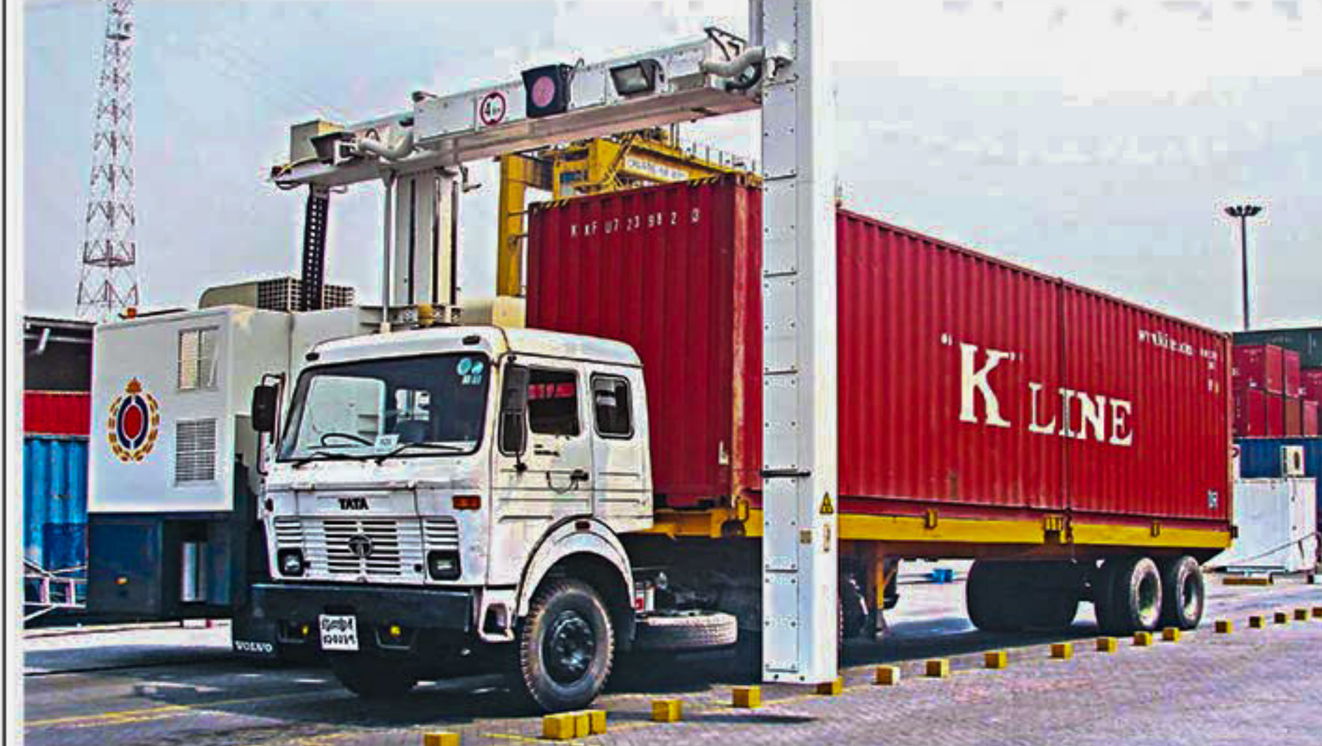
A container-laden truck passes through a scanner. The scanners reduce requirement for physical examination of shipment, bring down clearance time, and curb tax evasion.
