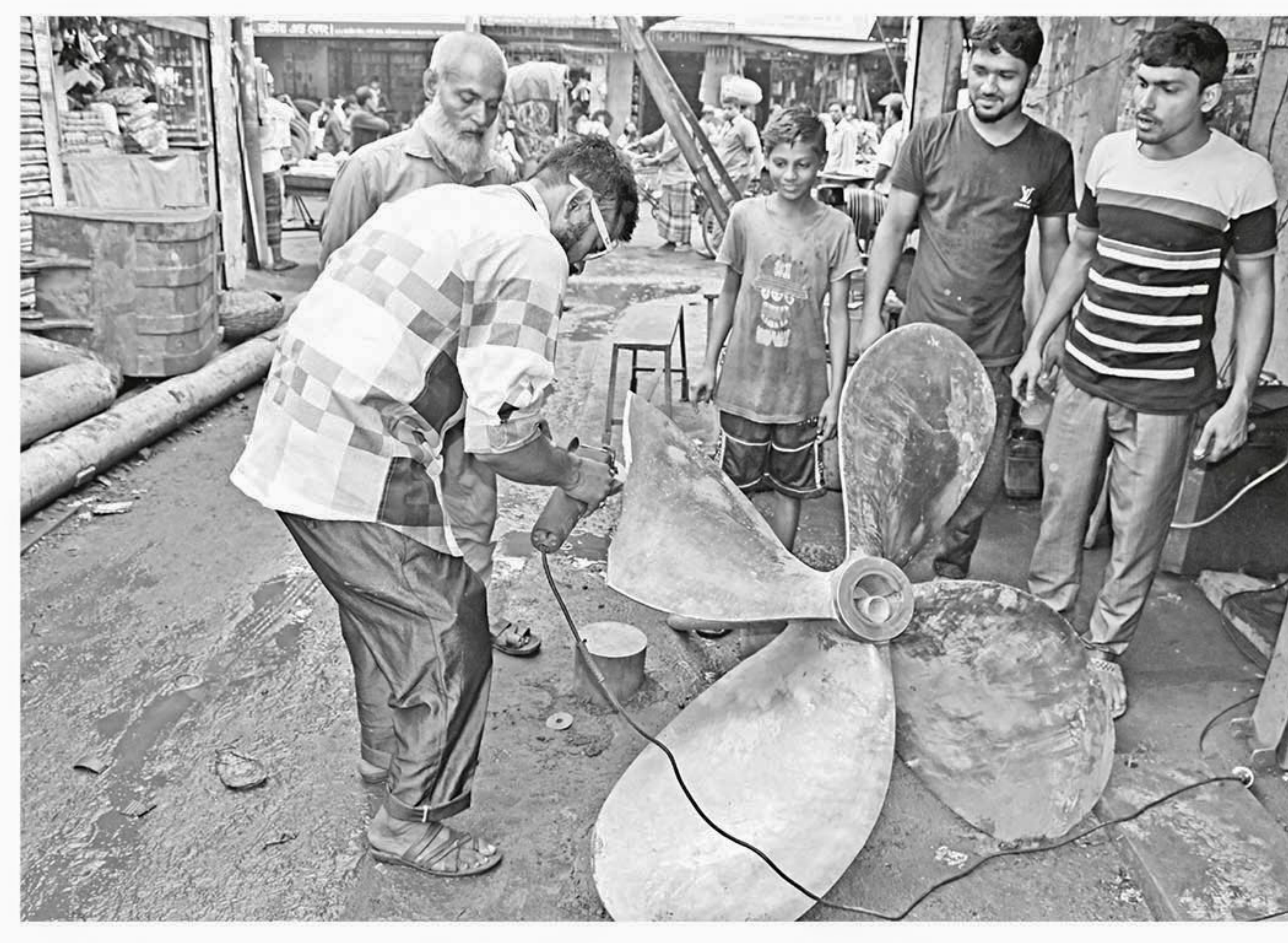
A worker repairs the broken blade of a cargo ship's propeller to later weld a replacement part into place. The photo was taken at Barishal city's Nasir Super Market yesterday. PHOTO: TITU DAS
