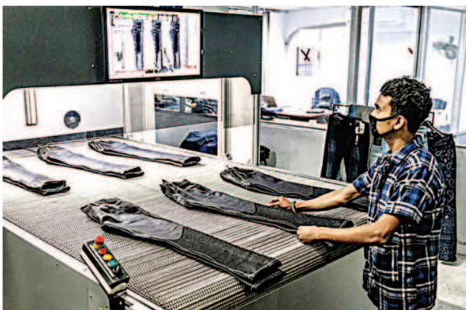
A worker uses a laser engraving machine to distress jeans at Denim Expert Ltd.
