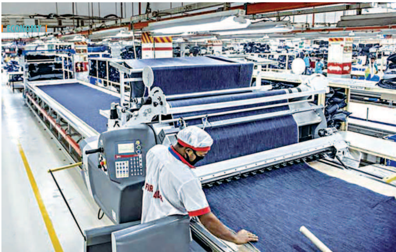
An automated spreading machine at Pacific Jeans.
