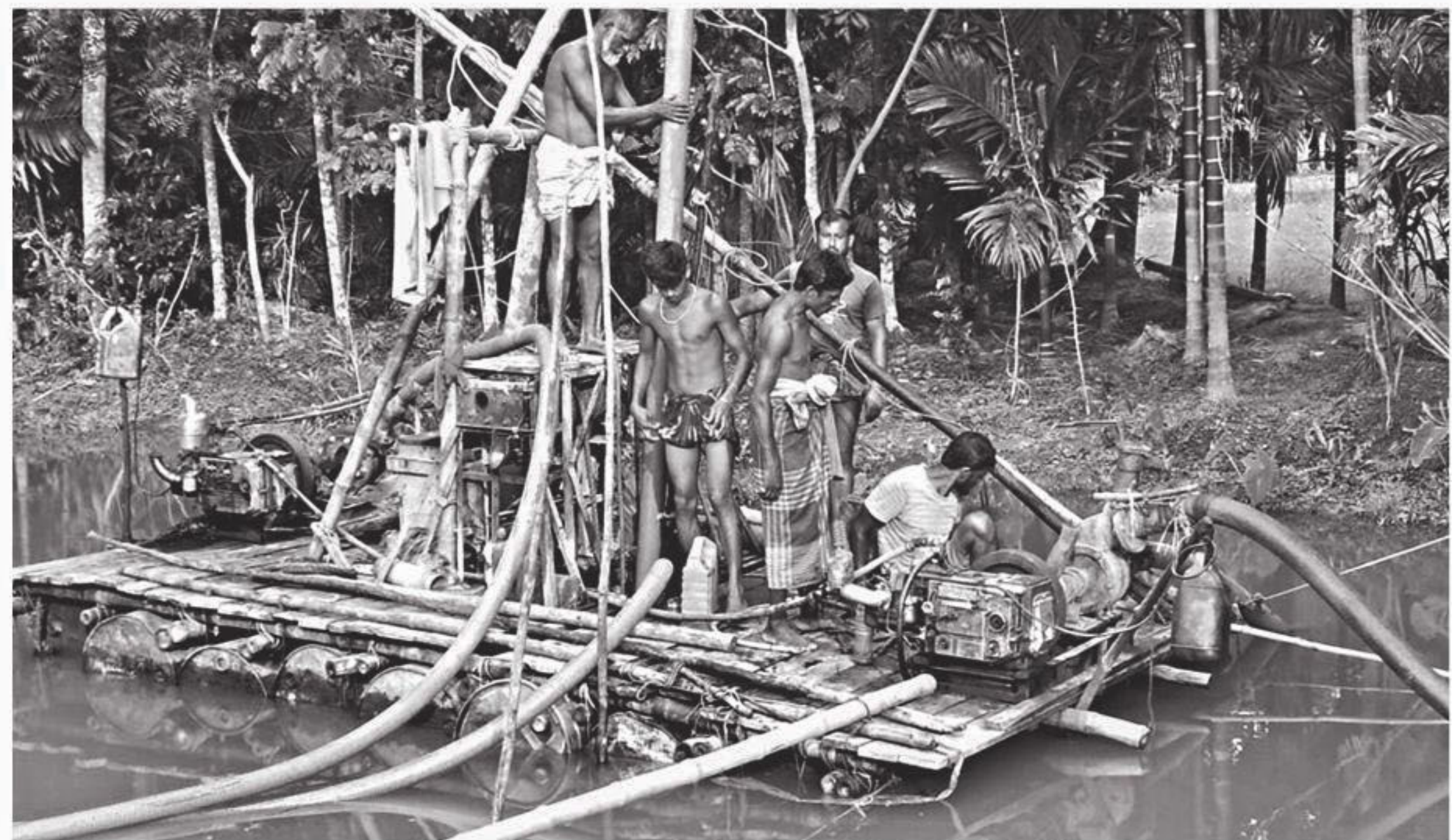
Labourers lift sand from a local water body with diesel-run shallow machine illegally in Tafalbari Bazar area in Sharankhola upazila of Bagerhat. PHOTO: STAR
