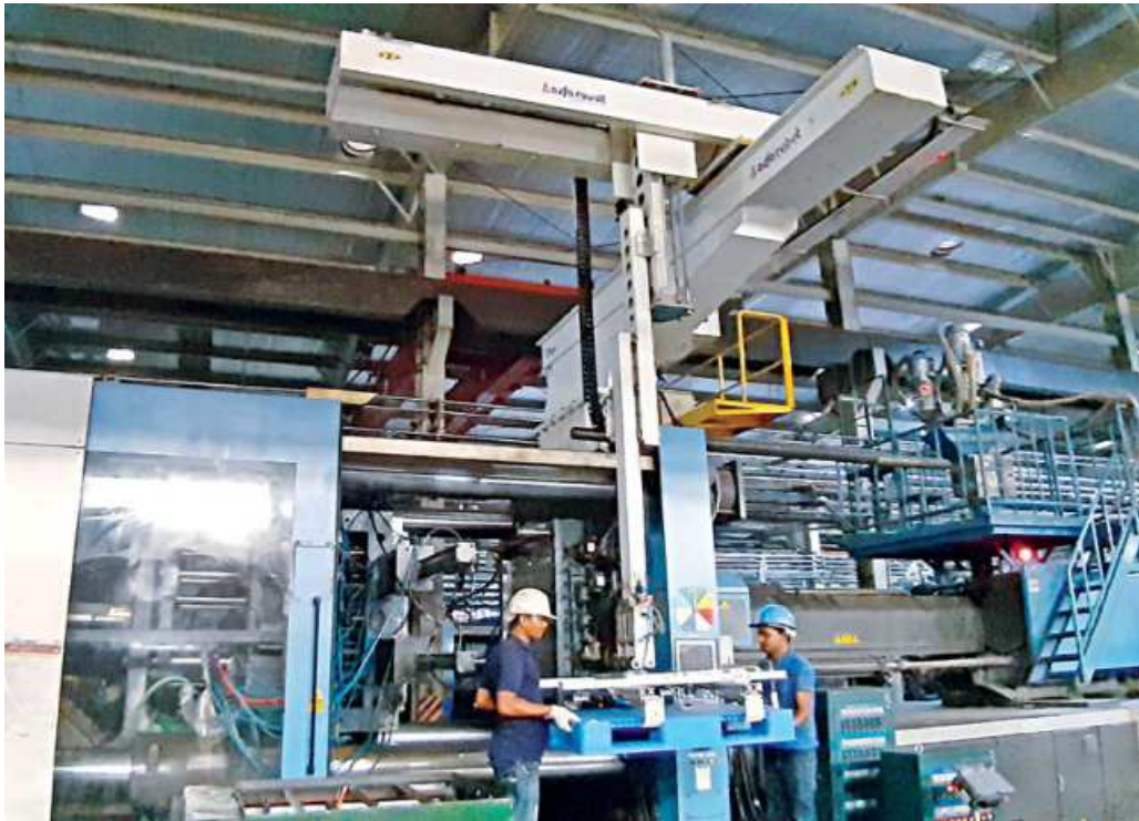
Robotic arms of an injection moulding machine are taking plastic pallets out of a mould at an RFL factory in Ghorashal, Narsingdi.
