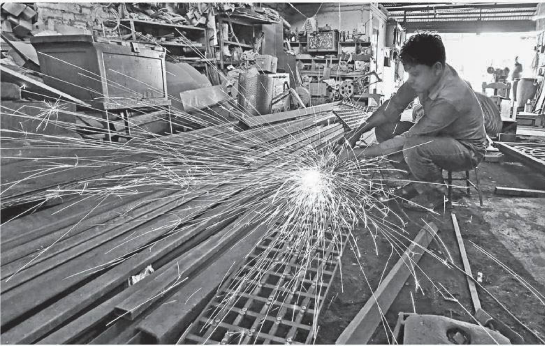
A worker grinds a metal gate inside a household furniture manufacturing factory in Ahmedabad, India.
