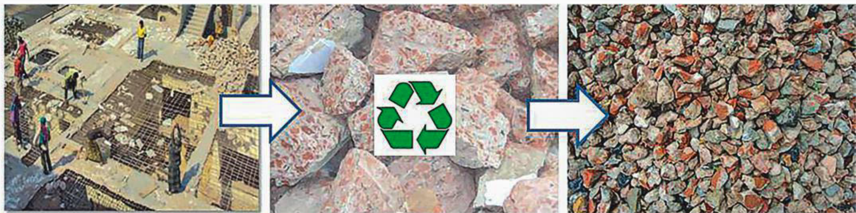
Recycling of demolished concrete waste as coarse aggregate for new construction works.
