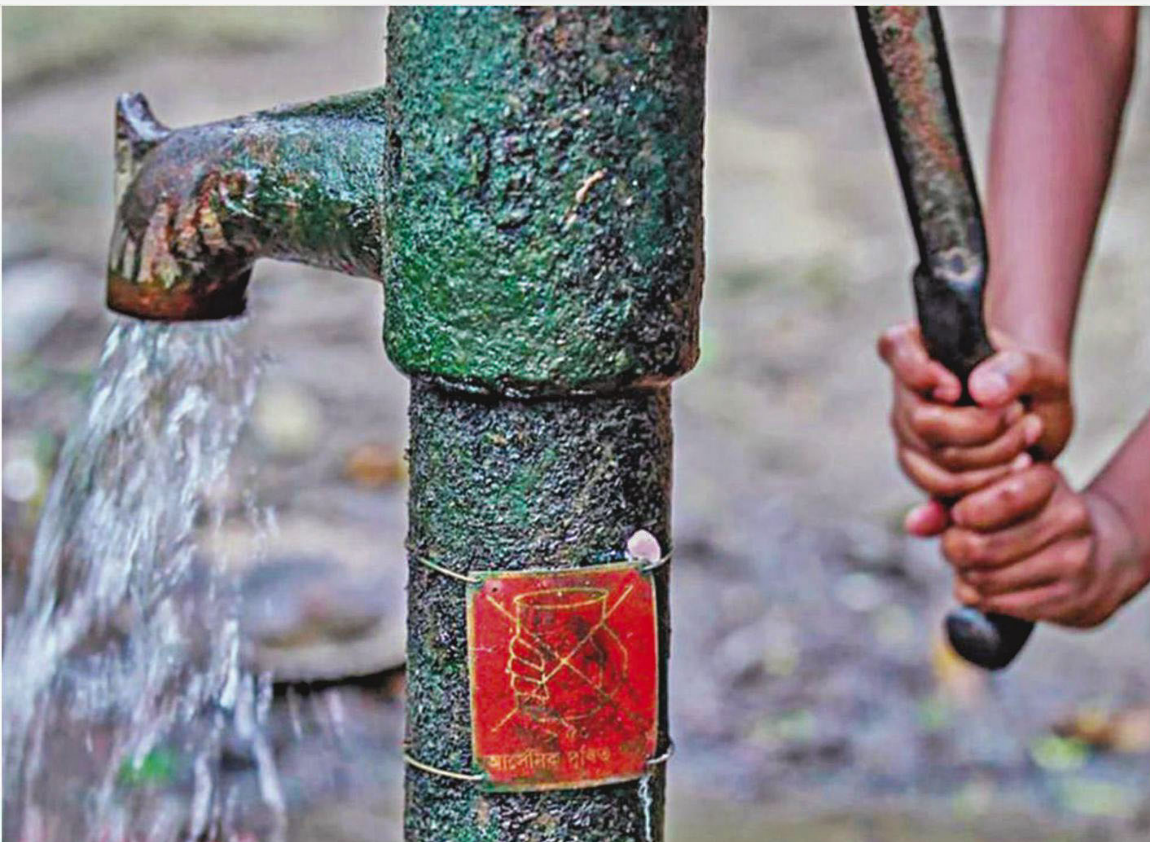
Red and green-painted tubewells have long since faded, with no further efforts made to distinguish unsafe wells from safe ones. PHOTO: STAR
