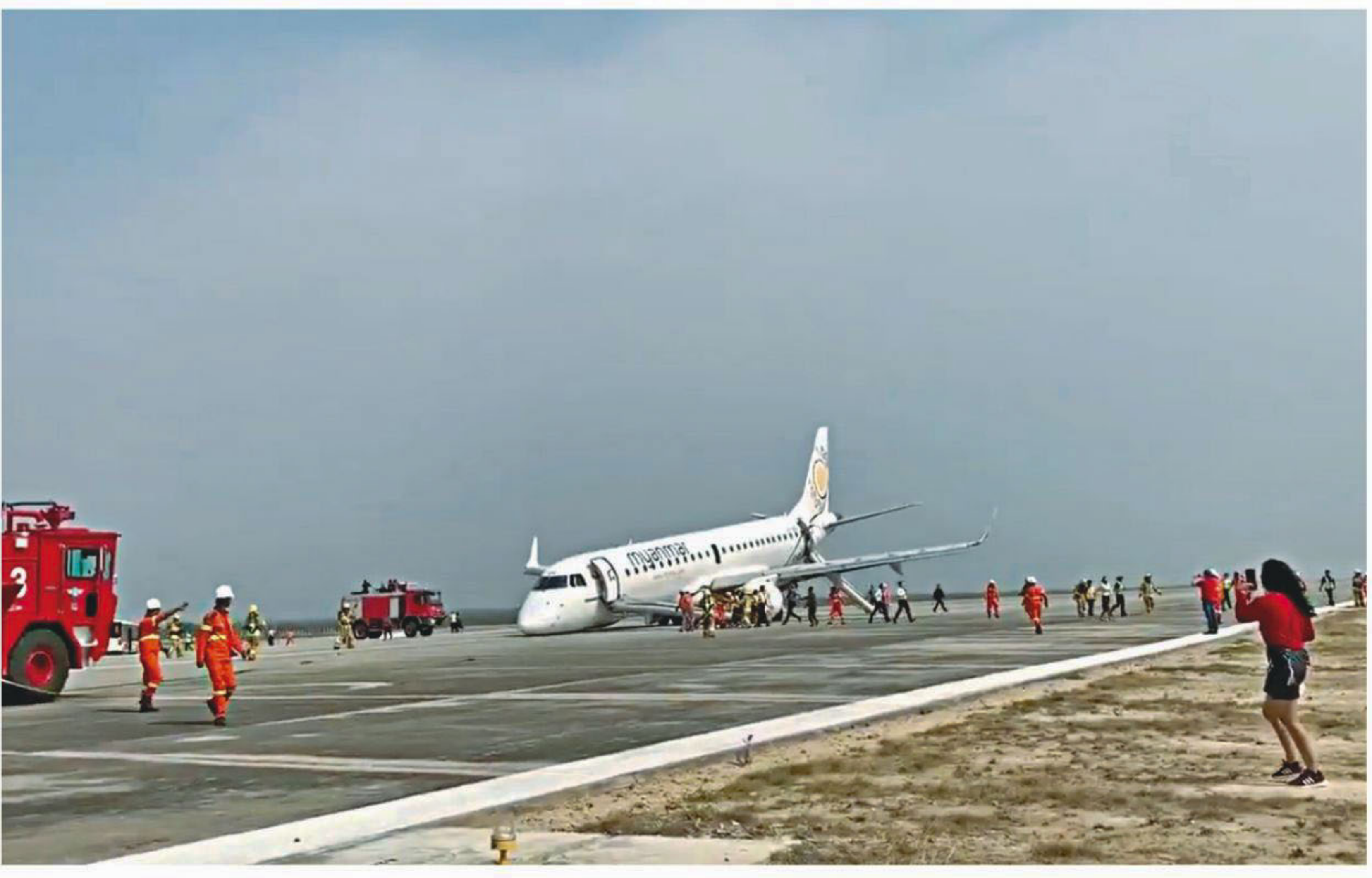
An evacuated passenger records on her phone as firefighters attend to the scene after Myanmar National Airlines flight UB103 landed without a front wheel at Mandalay International Airport in Tada-U, Myanmar yesterday in this still image taken from social media video. PHOTO: REUTERS
