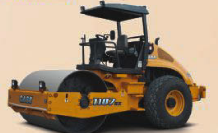
Vibratory Soil Compactor
