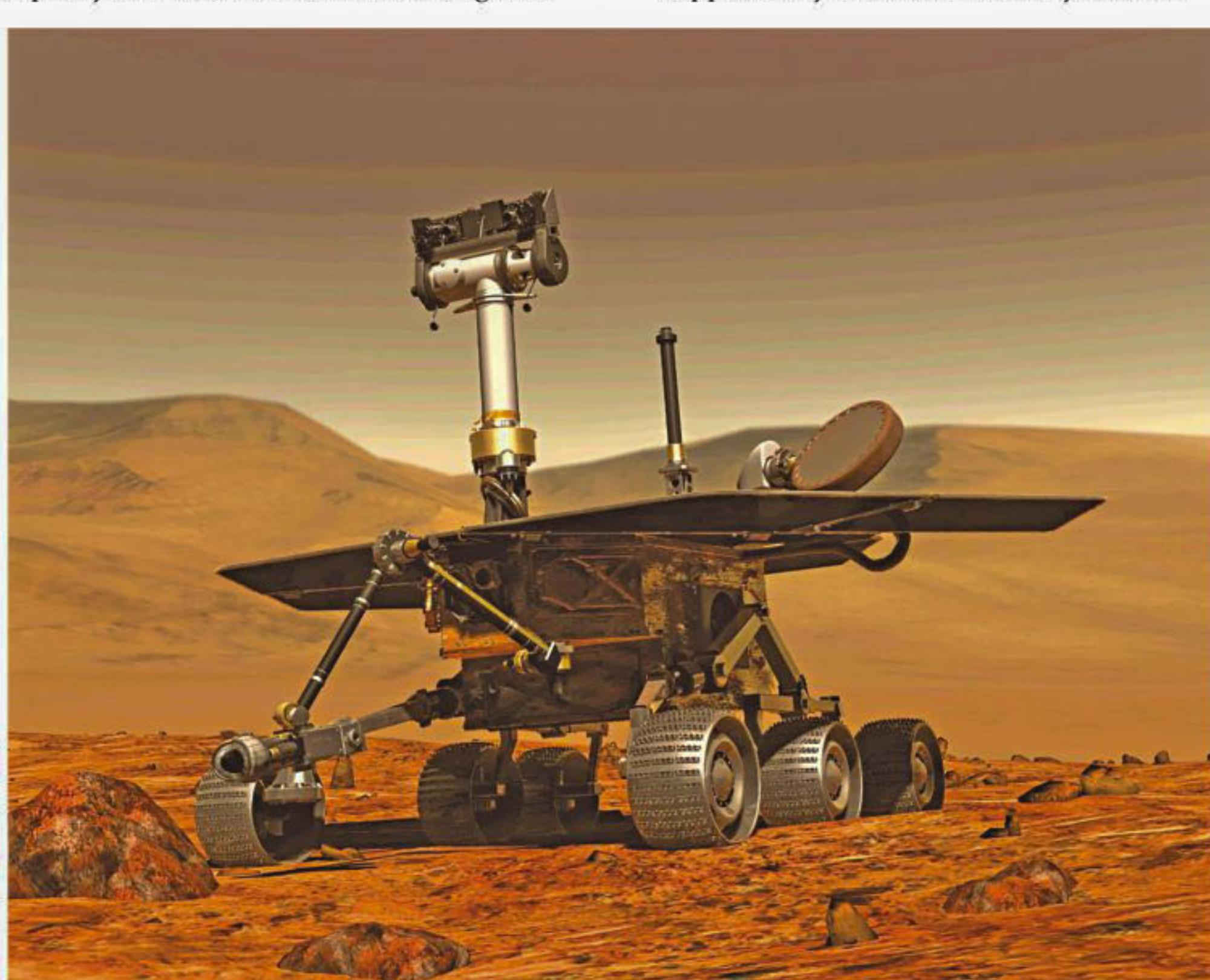
storm had finally hit. And the rover would have probably survived this dust storm too had it not been for Oppy's glitched heater. The heater on Oppy's robotic arm had been stuck in the "on" position ever since it landed on Mars and for all these years, scientists at NASA would have to shut down everything on the rover, even the crucial survival heaters every night so that its one bad heater wouldn't drain away crucial bat-
