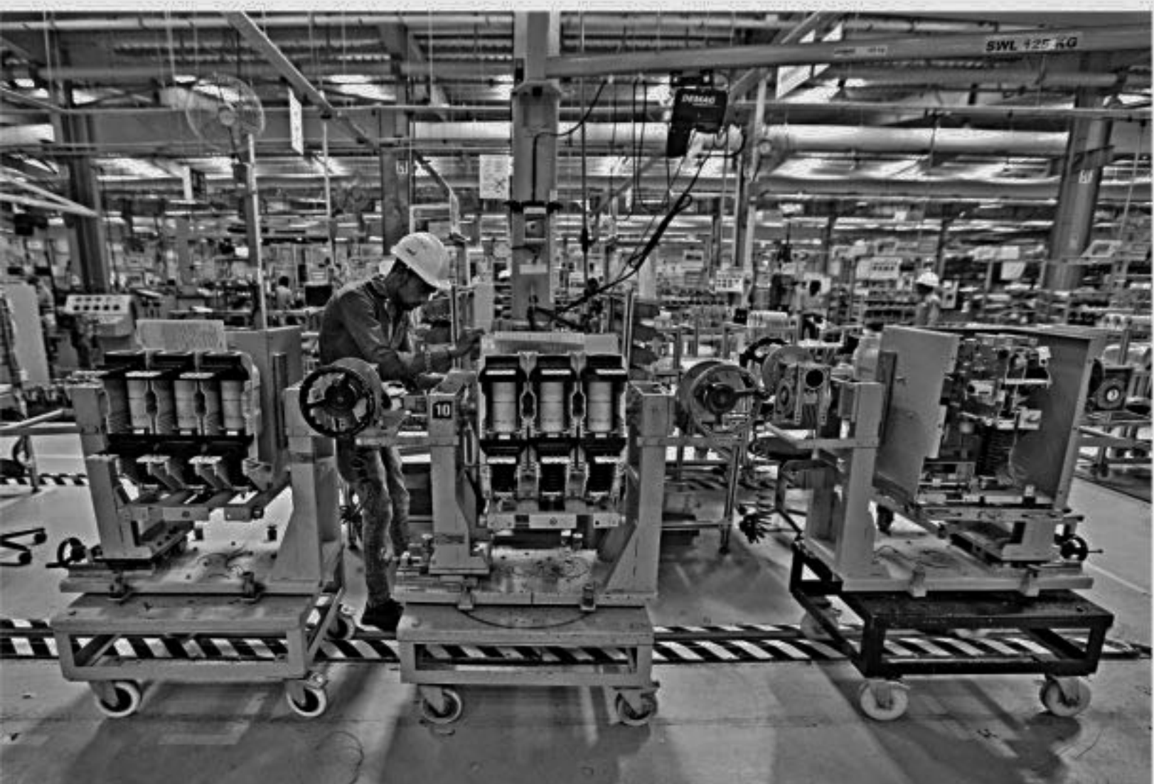
An employee assembles medium voltage switchgears inside a plant of a company in Gujarat.
