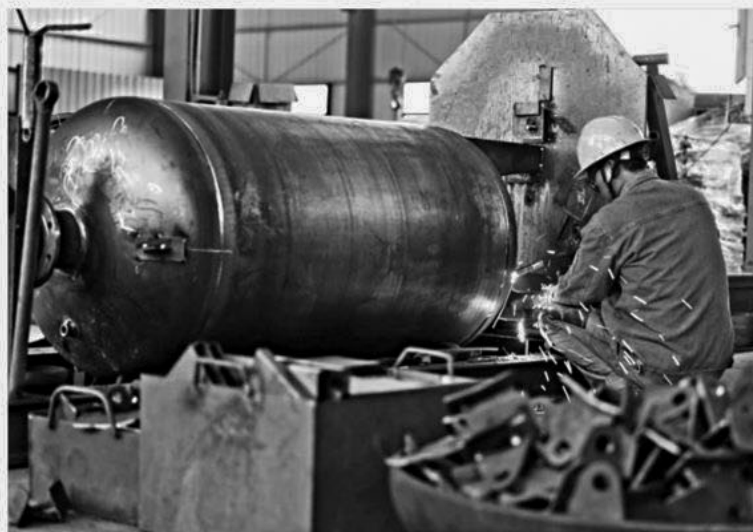
A worker welds a pressure vessel at a company manufacturing industrial equipment in China.
