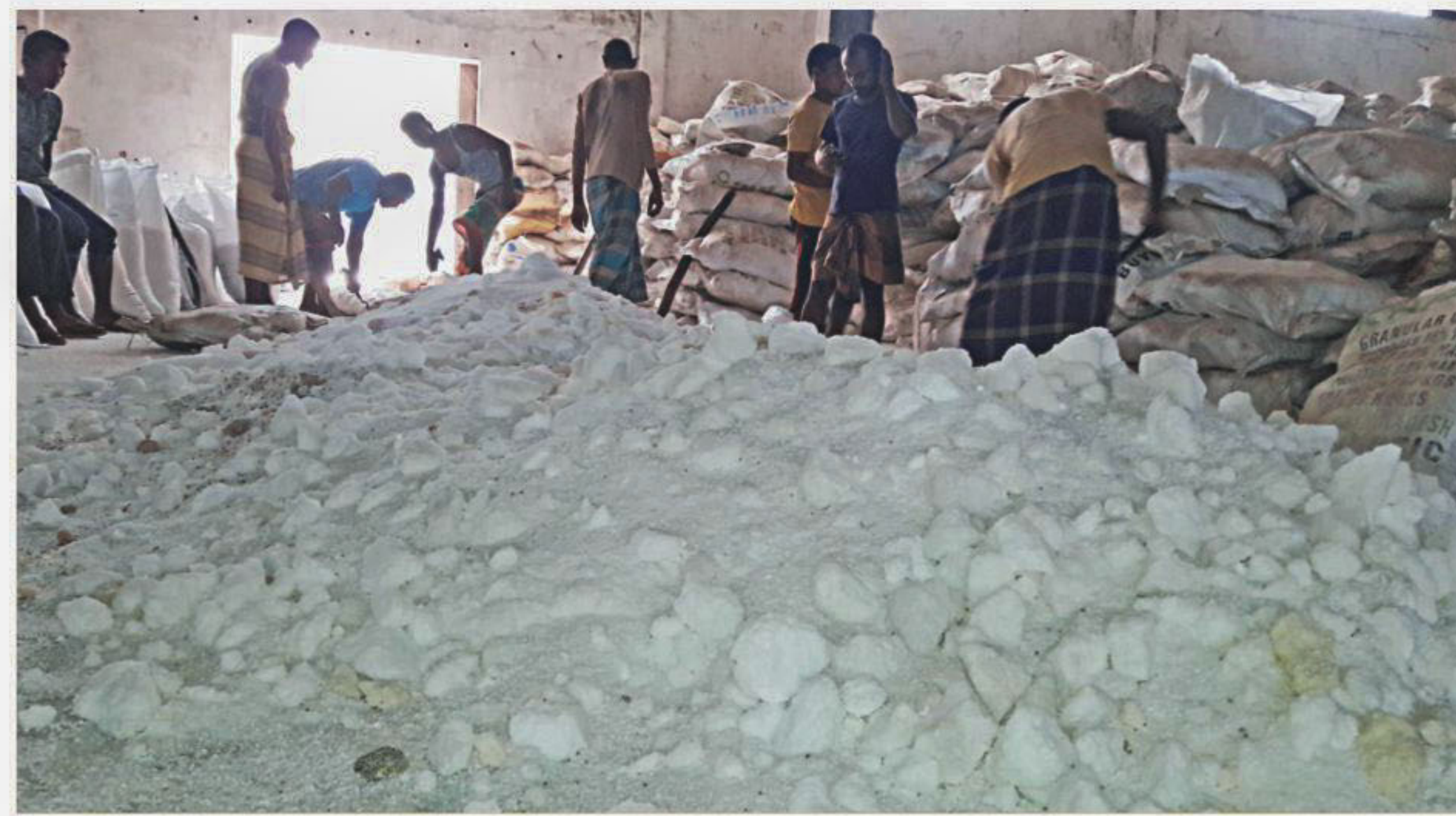
Workers crush coagulated urea fertiliser to repack it at the buffer godown of Bangladesh Chemical Industries Corporation at Mahendranagar in Lalmonirhat Sadar upazila. Around 1100 tonnes of fertiliser imported from China has reportedly turned solid at the warehouse, making the item unacceptable to dealers. PHOTO: S DILIP ROY
