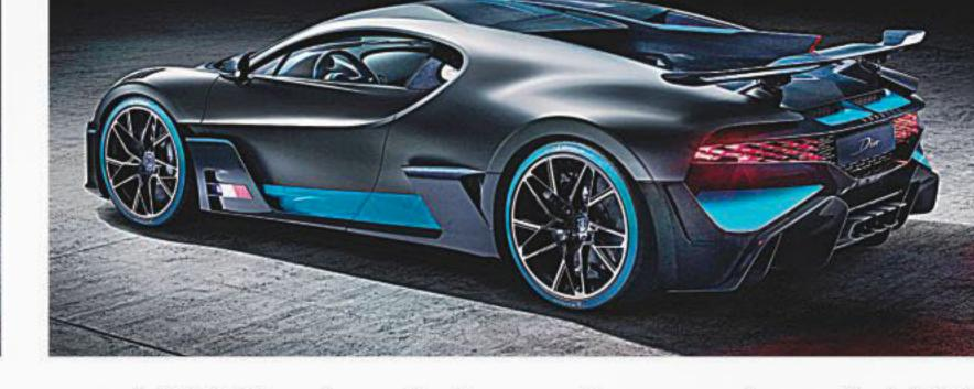
power - 1,479 HP from the quad turbo 8.0 litre W16 that powers the Chiron. The big difference comes in the aero while the Chrion was built for top speed and maximum slipperiness, the Divo's corner friendly aero produces 1,005 lbs of downforce in total. Top
