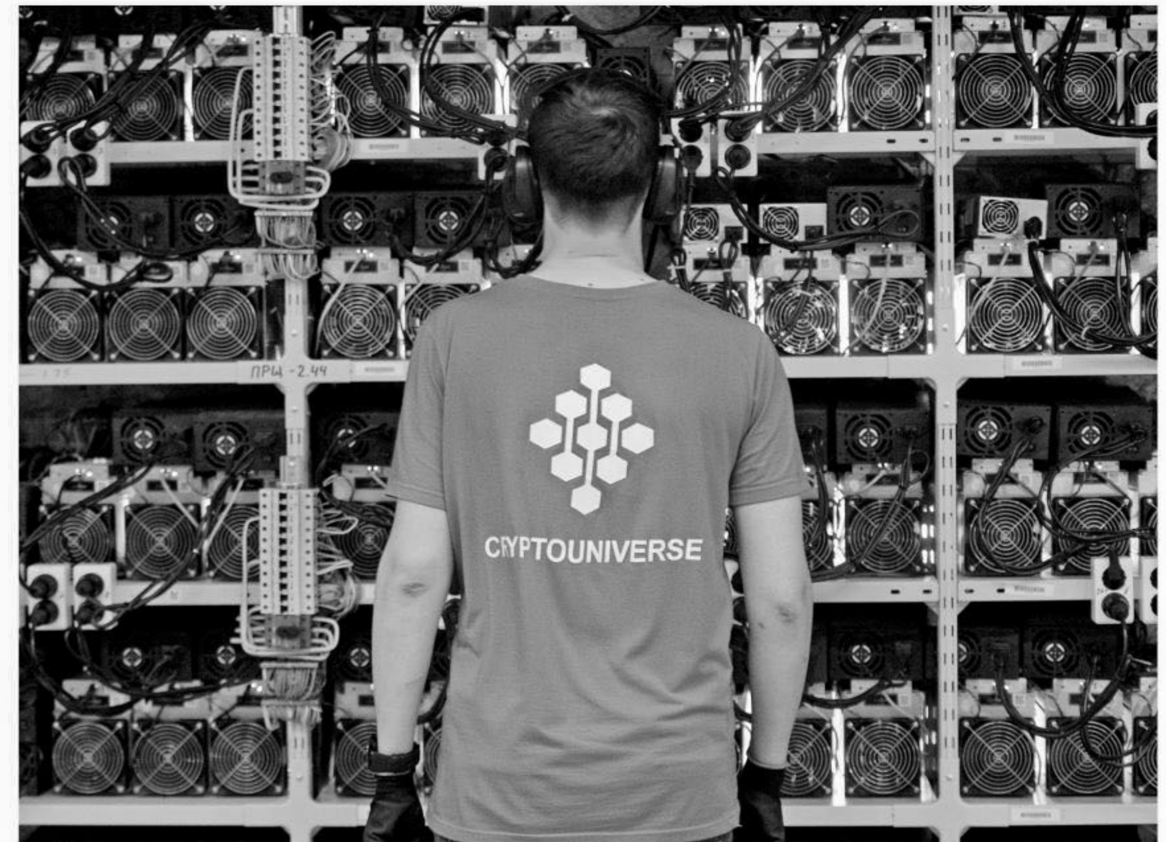
An employee inspects machines for the production of bitcoins and lightcoins at a mining centre in Russia.
