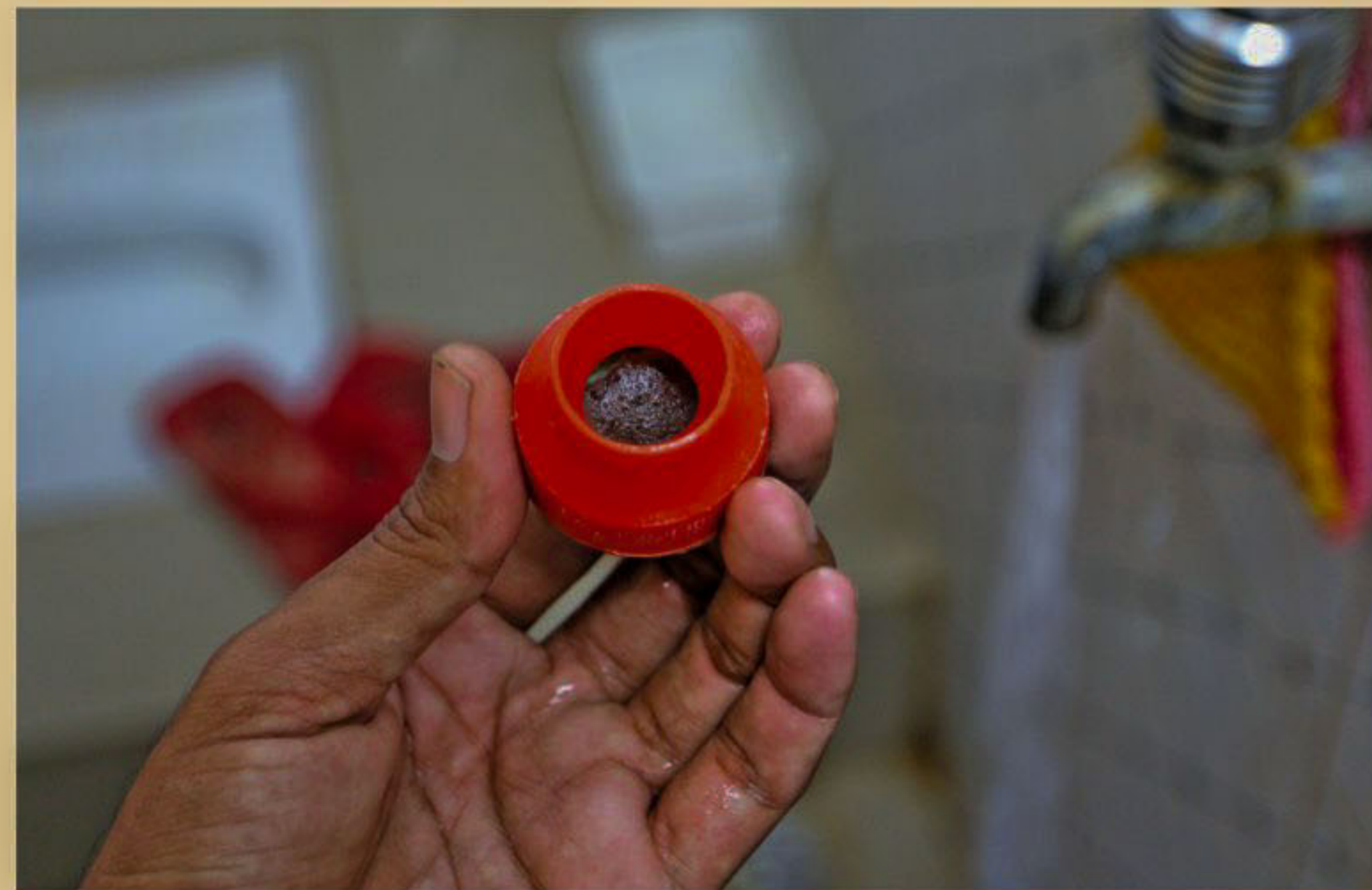
White filter turned pitch black moments after placing it under the water supplied by CWASA.
