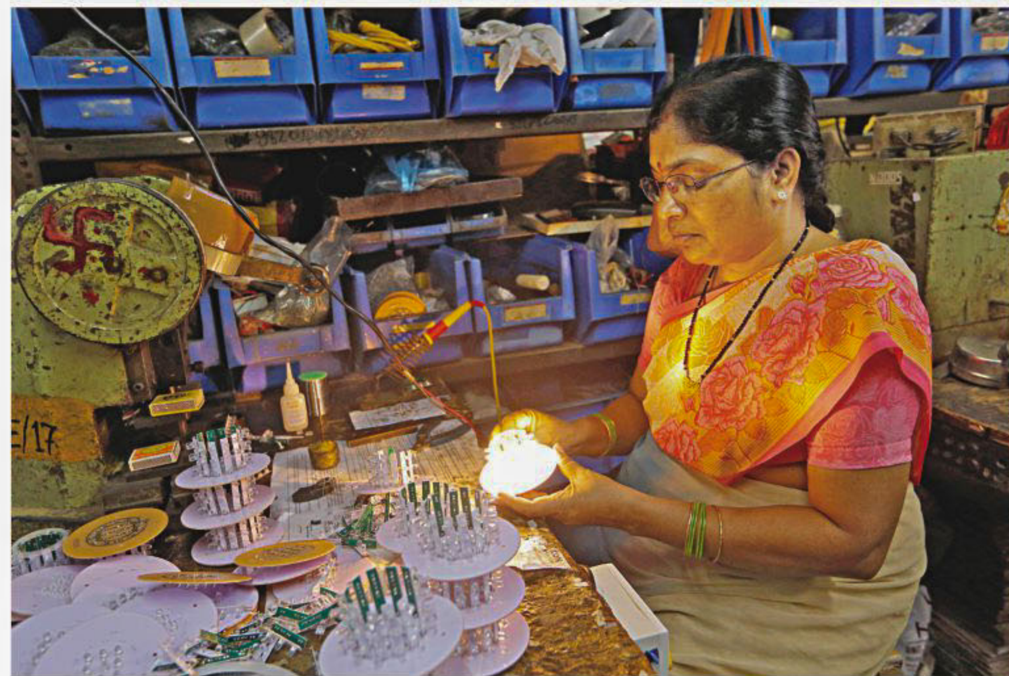
A woman tests LED bulbs after installing them onto a grid to make indicator lights inside an electrical manufacturing unit in Mumbai.
