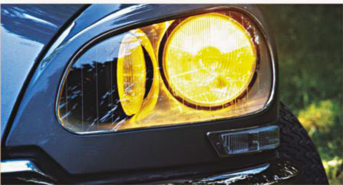
Citroen DS pioneered many things that boggle the minds of car manufacturers even today, like swiveling lights.
