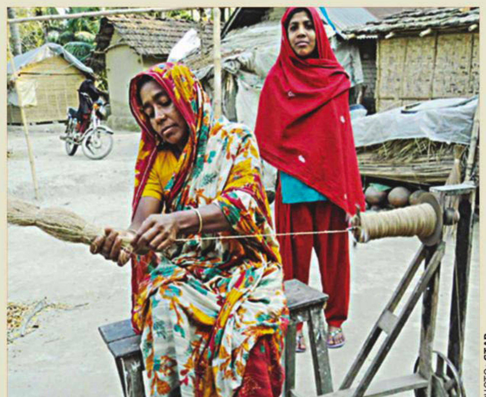
A good number of village women in Jessore's Monirampur upazila are engaged in making traditional coir ropes using fibre of coconut shells.
