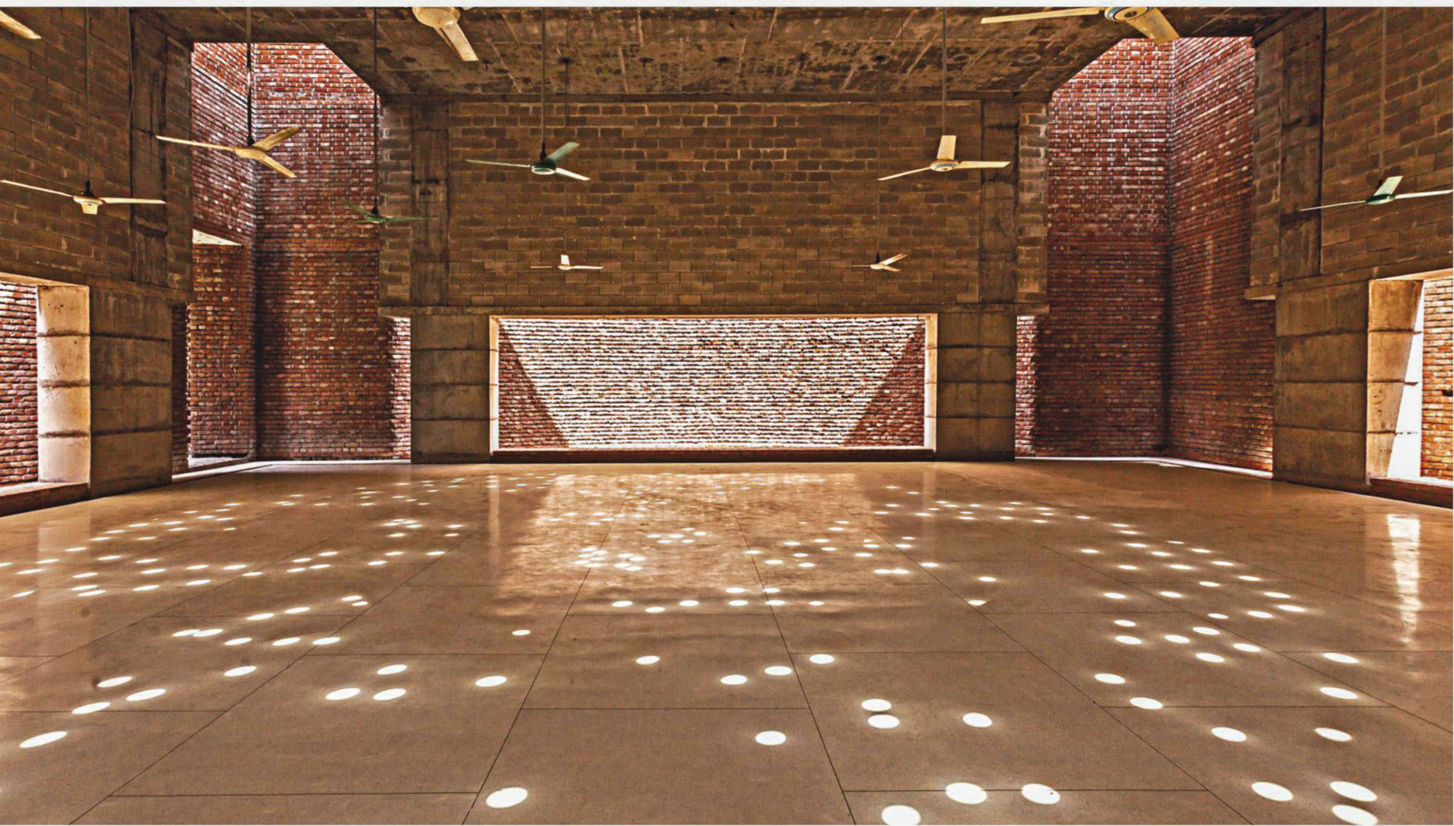
In addition to four light courts, random circular roof openings allow daylight into the prayer hall creating an ornate pattern on the floor enhancing spirituality through light. Baifur Mosque, Dhaka, Bangladesh, designed by Marina Tabassum.
