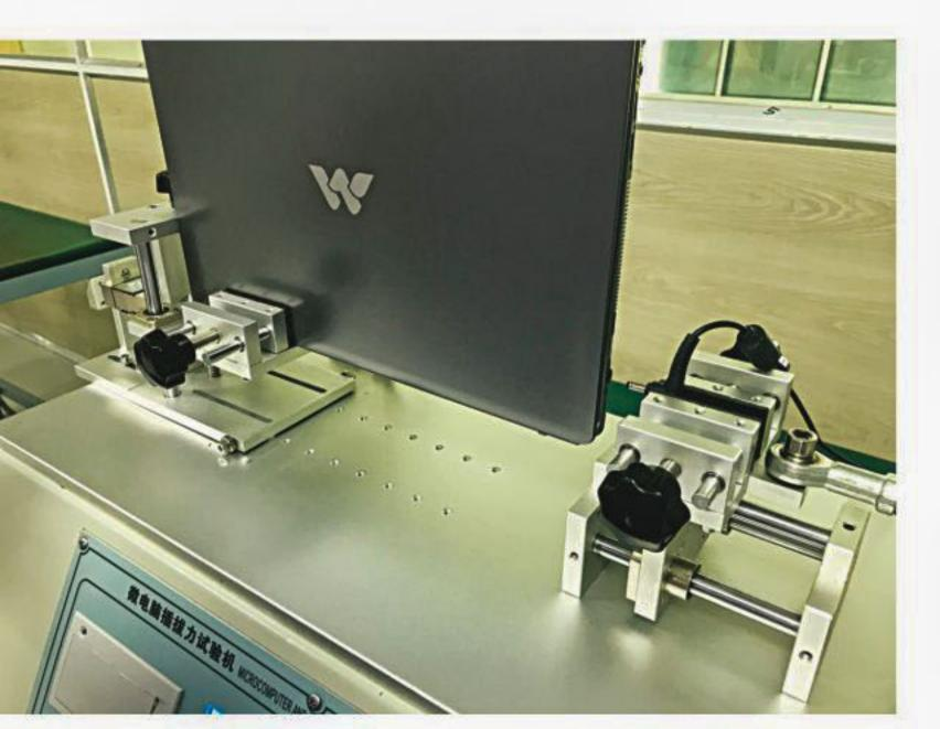
The LCD panel of the laptop does need to pass a hefty quality check in order to make its way to the market. Here the mechanised pressure tool checks if the display panel is properly fitted or not.
