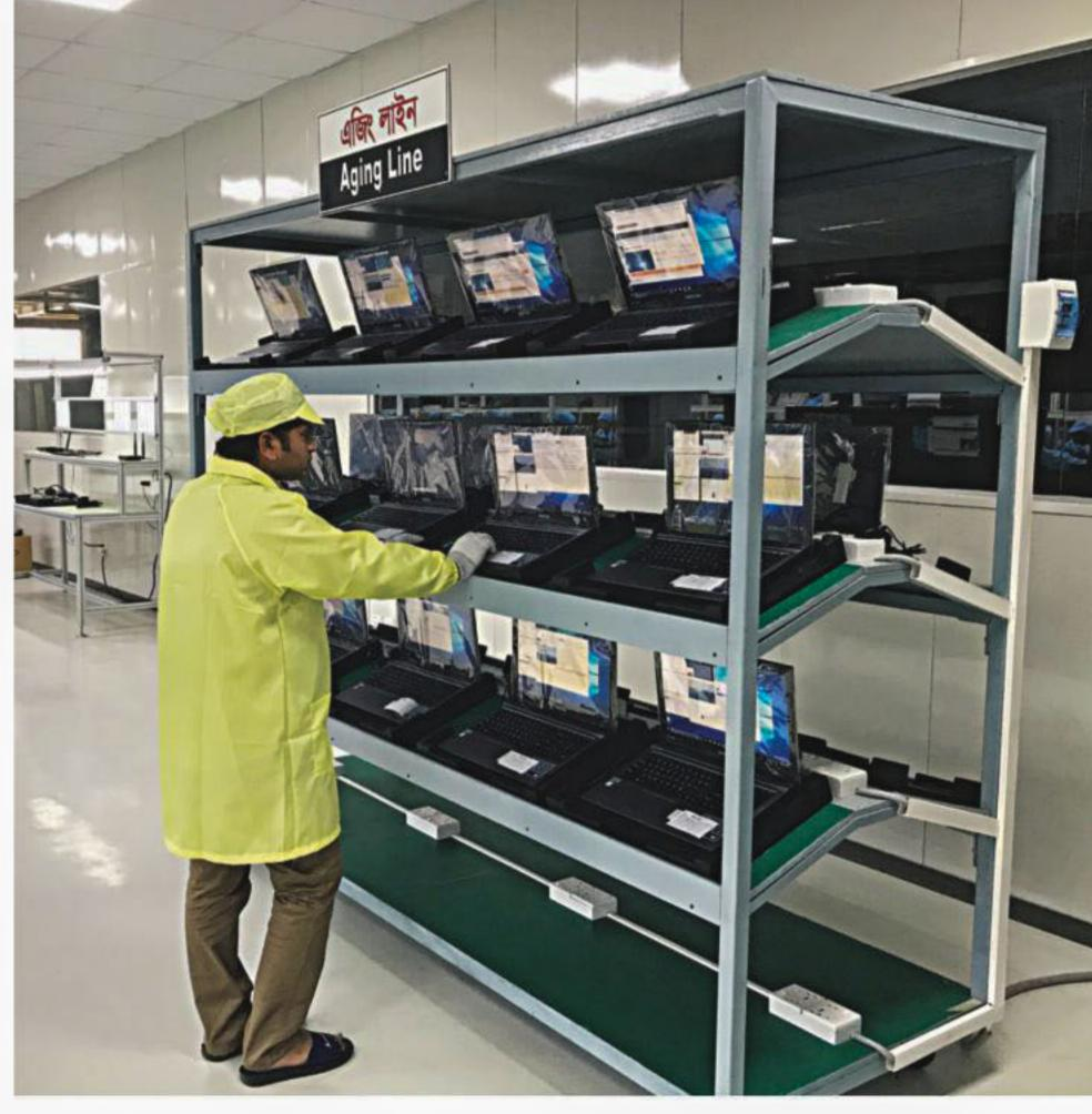
After a batch of laptops are assembled, they undergo intensive quality and performance testing. The quality assurance is of global standard before any laptop gets green signal,
