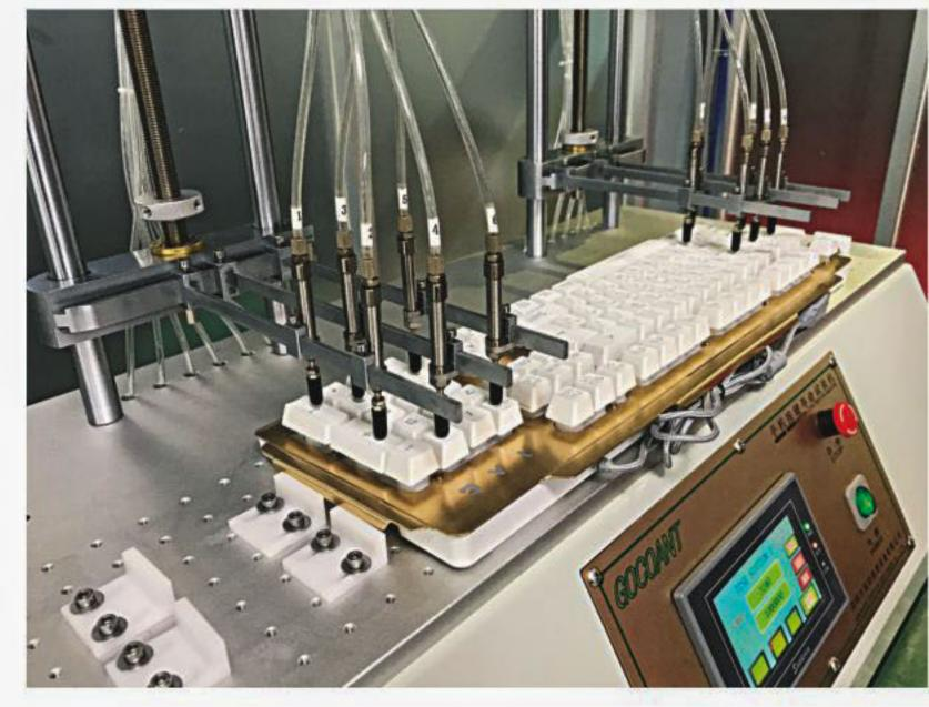
This is where the keyboards undergoes testing. These long poking machines are able to mimic human fingers. In a matter of minutes, the machine can do several thousands of keystrokes.
