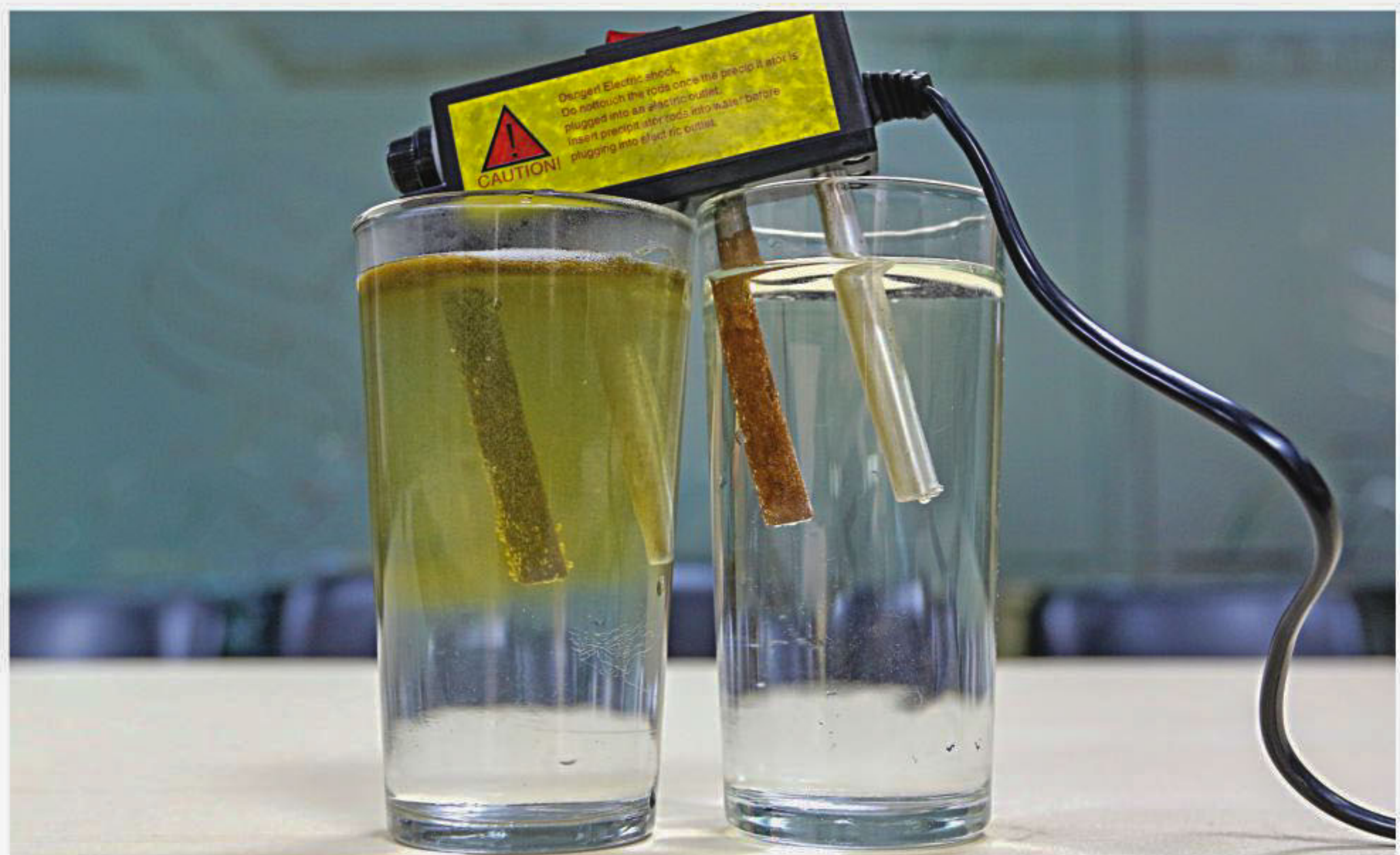
The electrolysis machine exposes the iron content in water. The water containing iron turns yellow after electrolysis.
