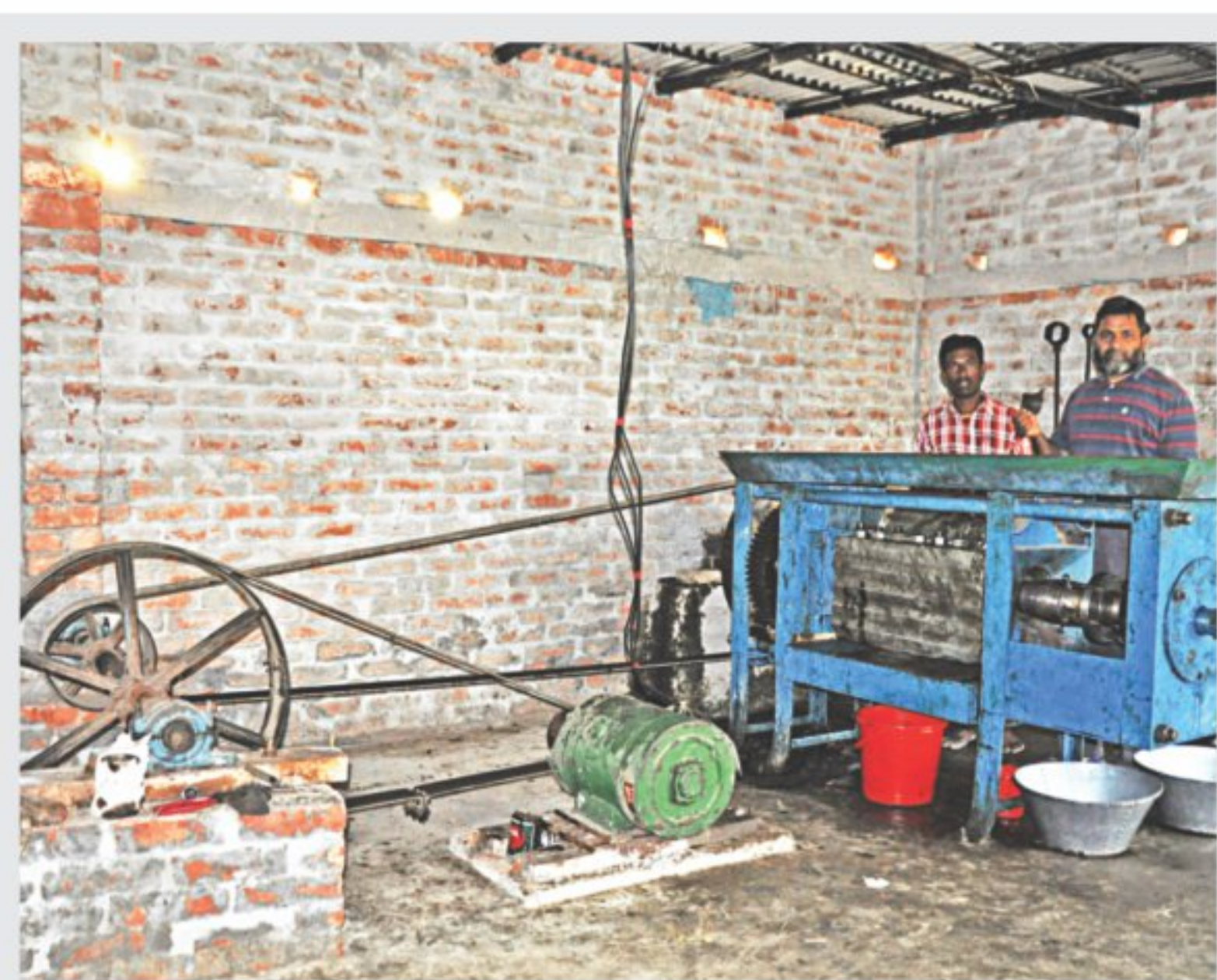
Linseed grinding machine run on solar minigrid power.
