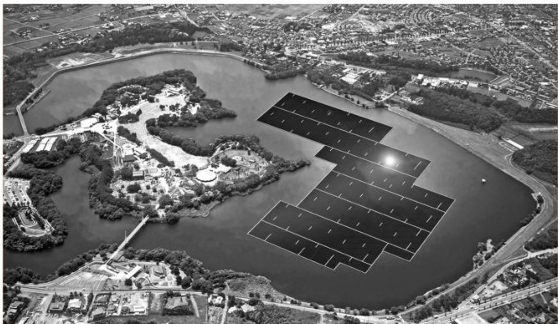
The 13.7 MW floating solar PV plant on Japan's Yamakura Dam reservoir, the largest installation of its kind in the world.
