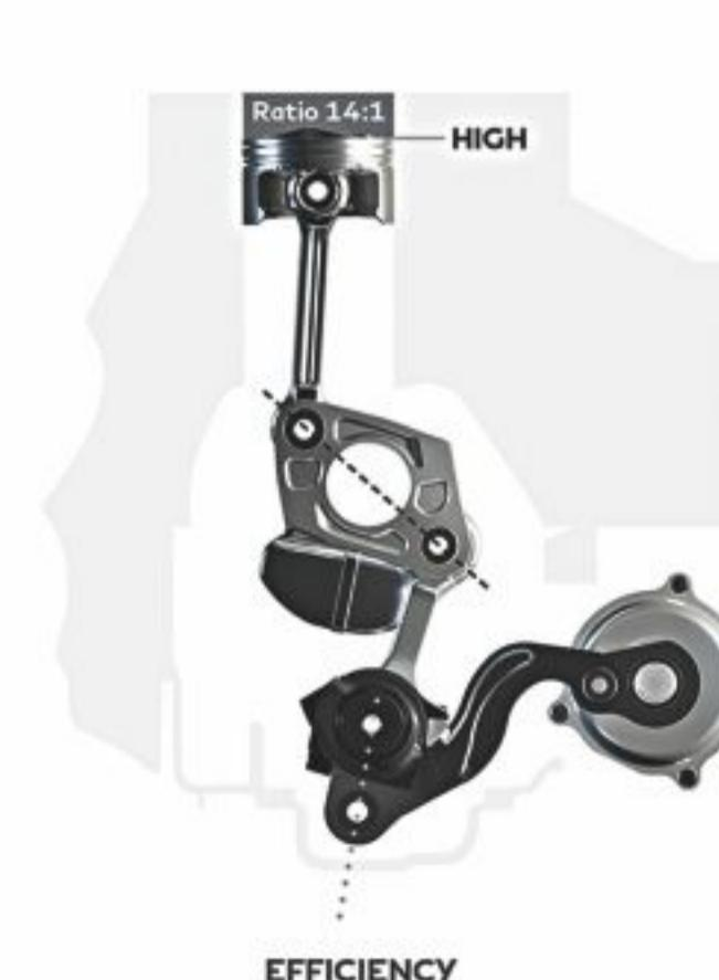
*During normal driving, efficiency is prioritised with a high compression ratio (the piston can reach higher up the combustion chamber and thus compress greater fuel and air before combustion occurs).*
