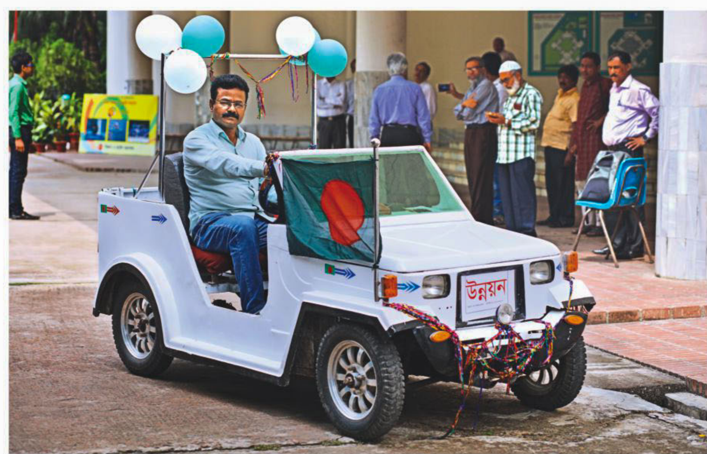
A 100CC CAR! Mizanur Rahman from Sharsha upazila of Jessore has built a car from a 100cc capacity engine of a motorcycle. His project won the first prize in a contest of the National Science and Technology Museum. The car can run 30-35km on a litre of octane. If the fuel runs out, the vehicle uses electricity. The photo of the car with Mizanur behind the wheel was taken in front of the museum yesterday.
