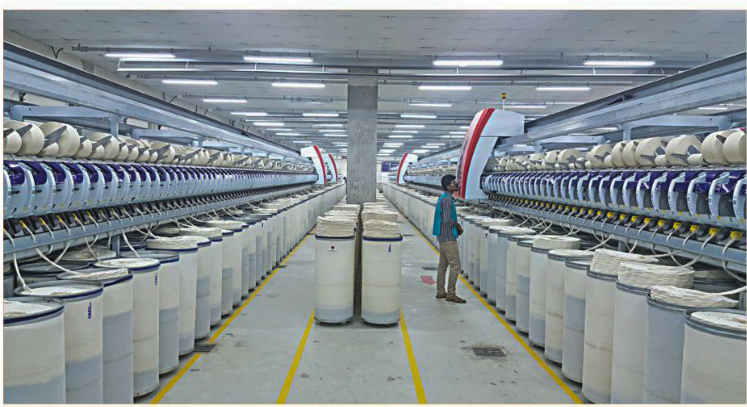
Autoconers process yarns at a factory of Envoy Textile, a spinning and denim fabrics manufacturer in Bhaluka. Autoconer is a robotic machine used in winding process to get high quality yarns with low manpower.
