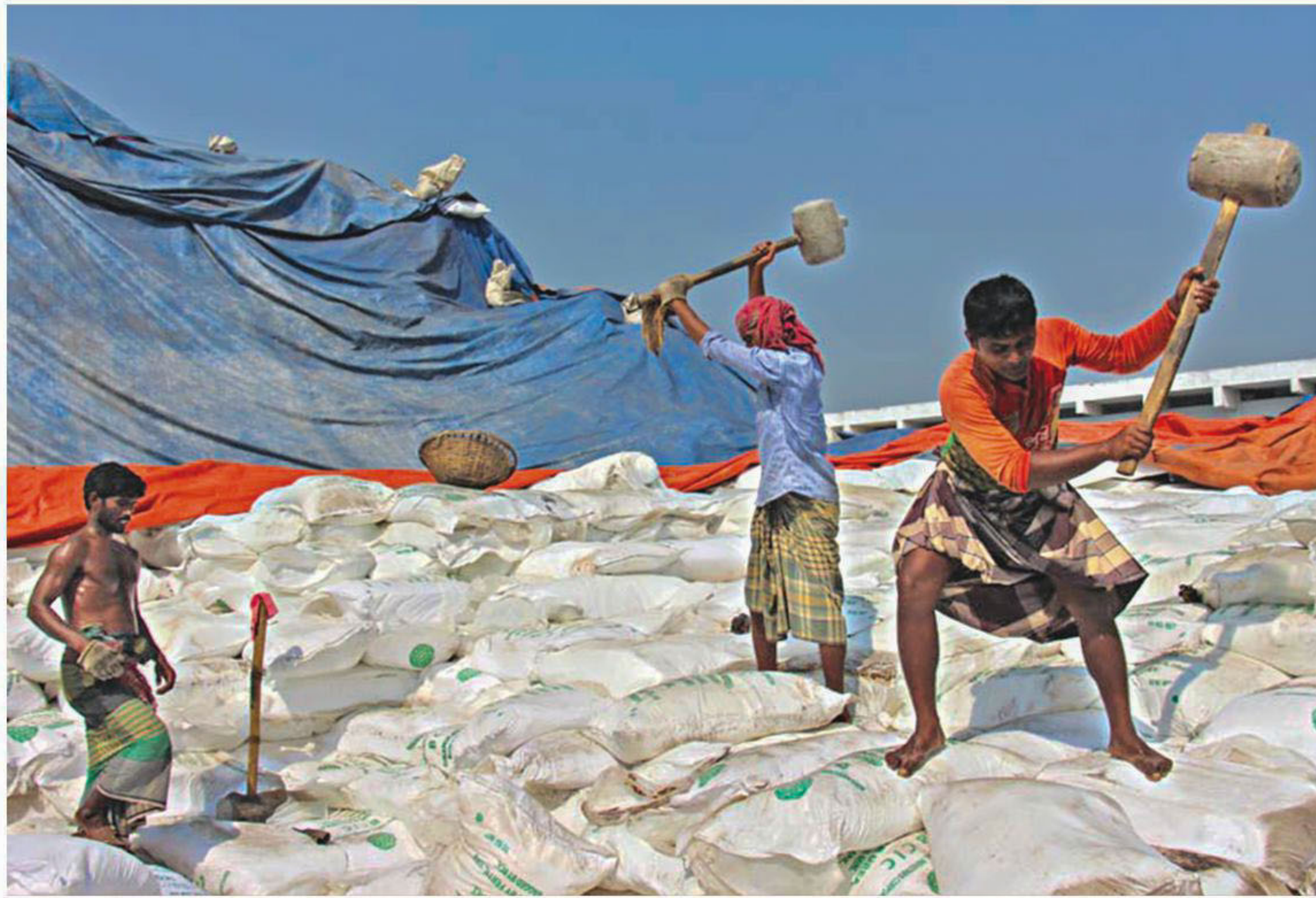
Workers hammering solidified sacks of fertiliser at Baghabari port in Sirajganj a couple of days ago. Later, the fertiliser grounds are distributed among farmers. The fertiliser turned solid as the sacks were kept in the open for months after import.
