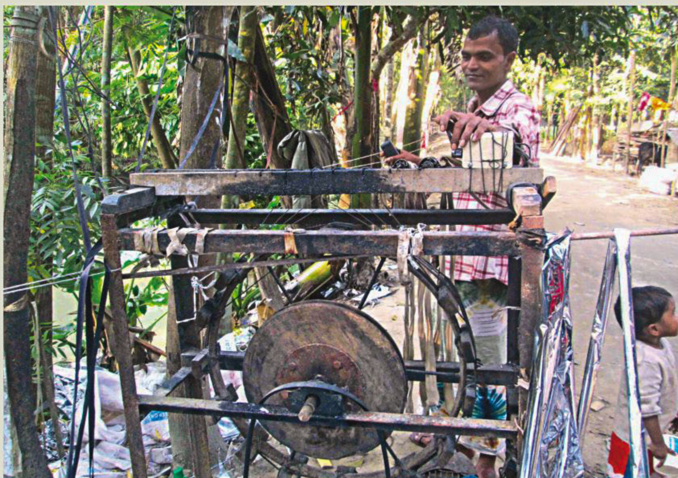
Jahid is busy producing rope from discarded polythene with his simple machine. The 36-year-old from Pirojpur spends Tk 32 to make 1kg rope that he sells at Tk 40 to wholesalers.
