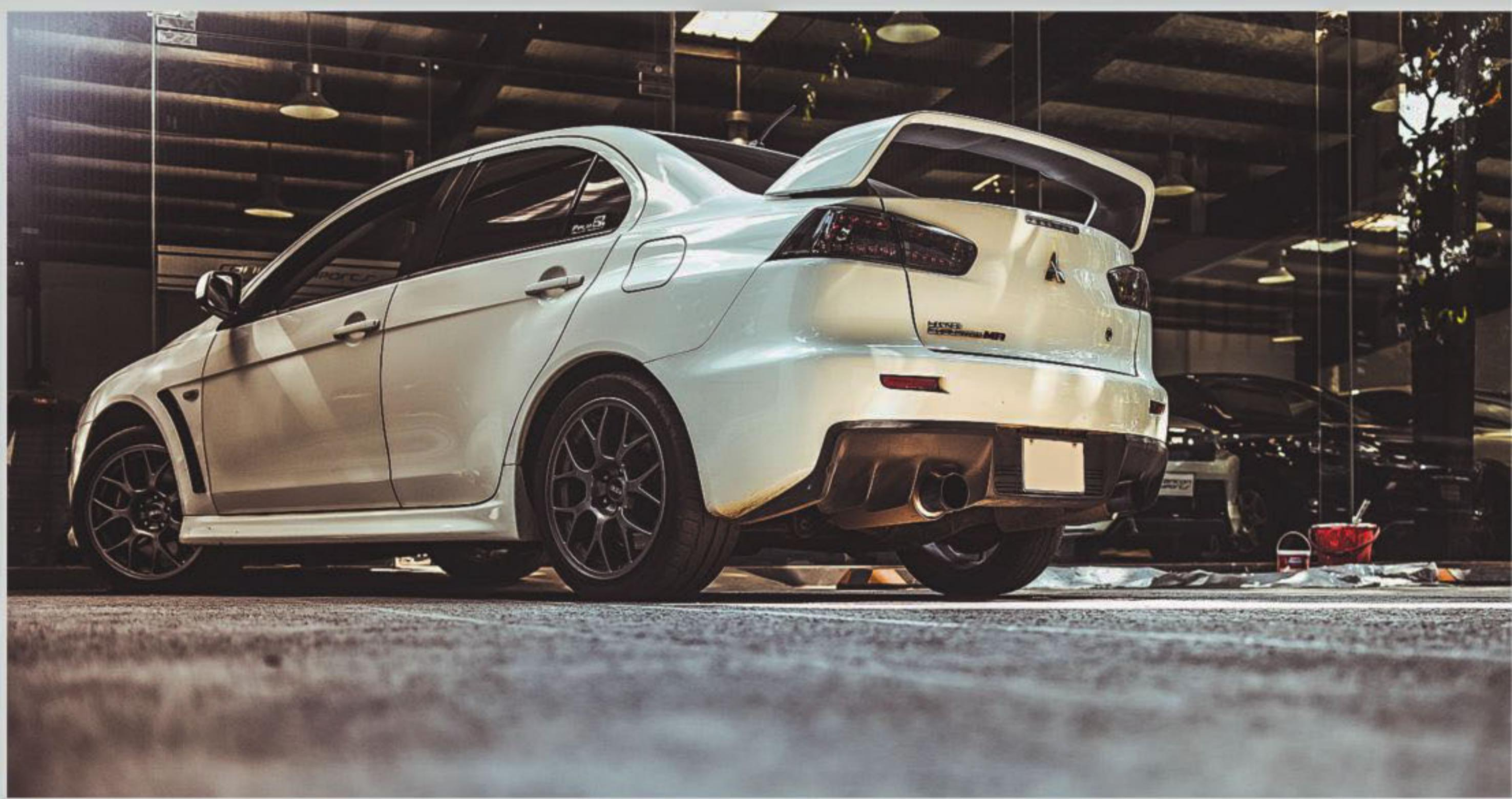
The Evolution X is apparently the last of the legendary Evo series, and it's the only Evo to be offered with a 6-speed Dual Clutch Automatic transmission, labeled the SST in the MR variant, which is supposedly faster than the manual GSR counterparts.
