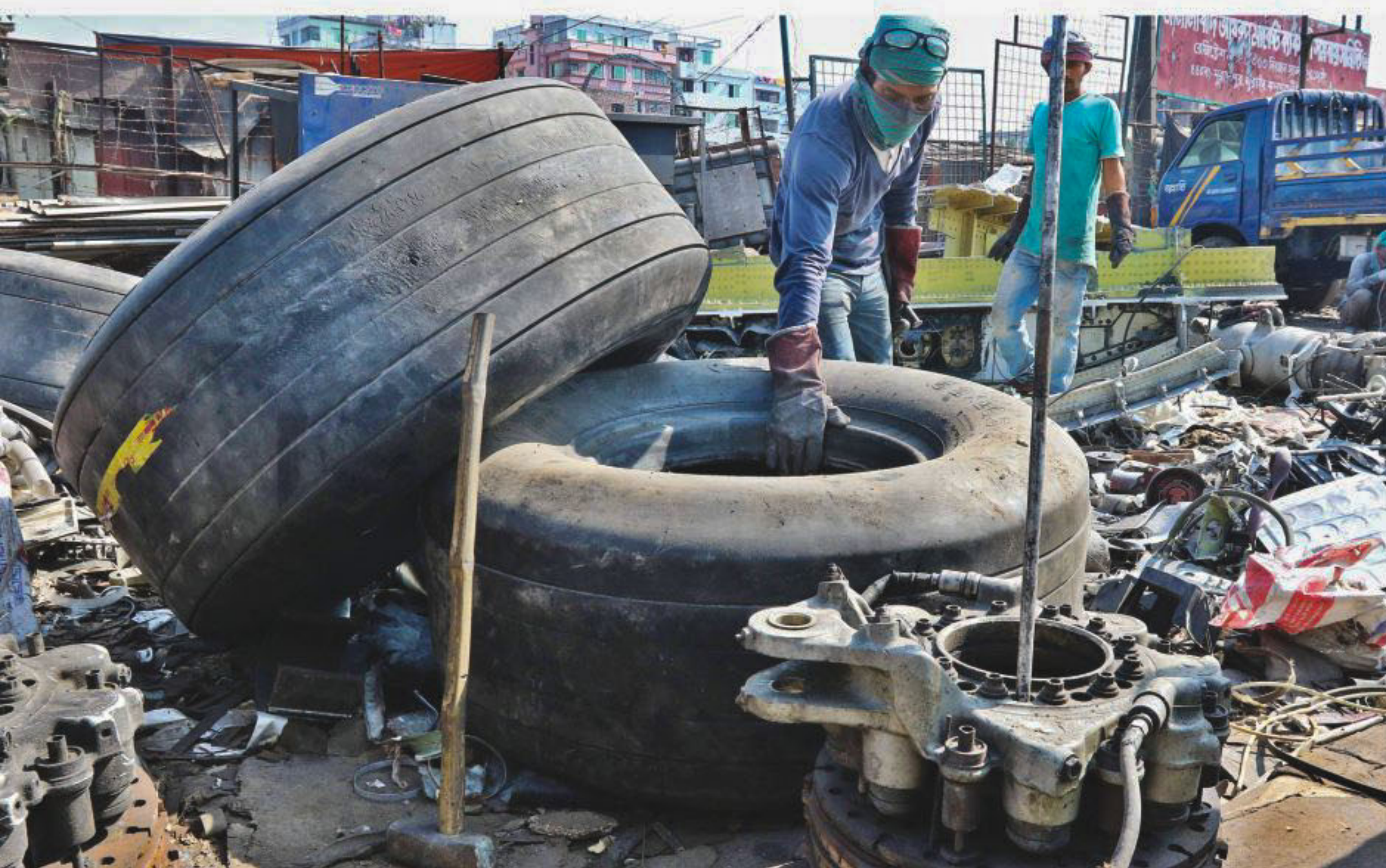
Tyres and disk brakes of a DC-10 are being taken away for melting and chunks of body is being cut into smaller bits to salvage the aviation-grade aluminium.
