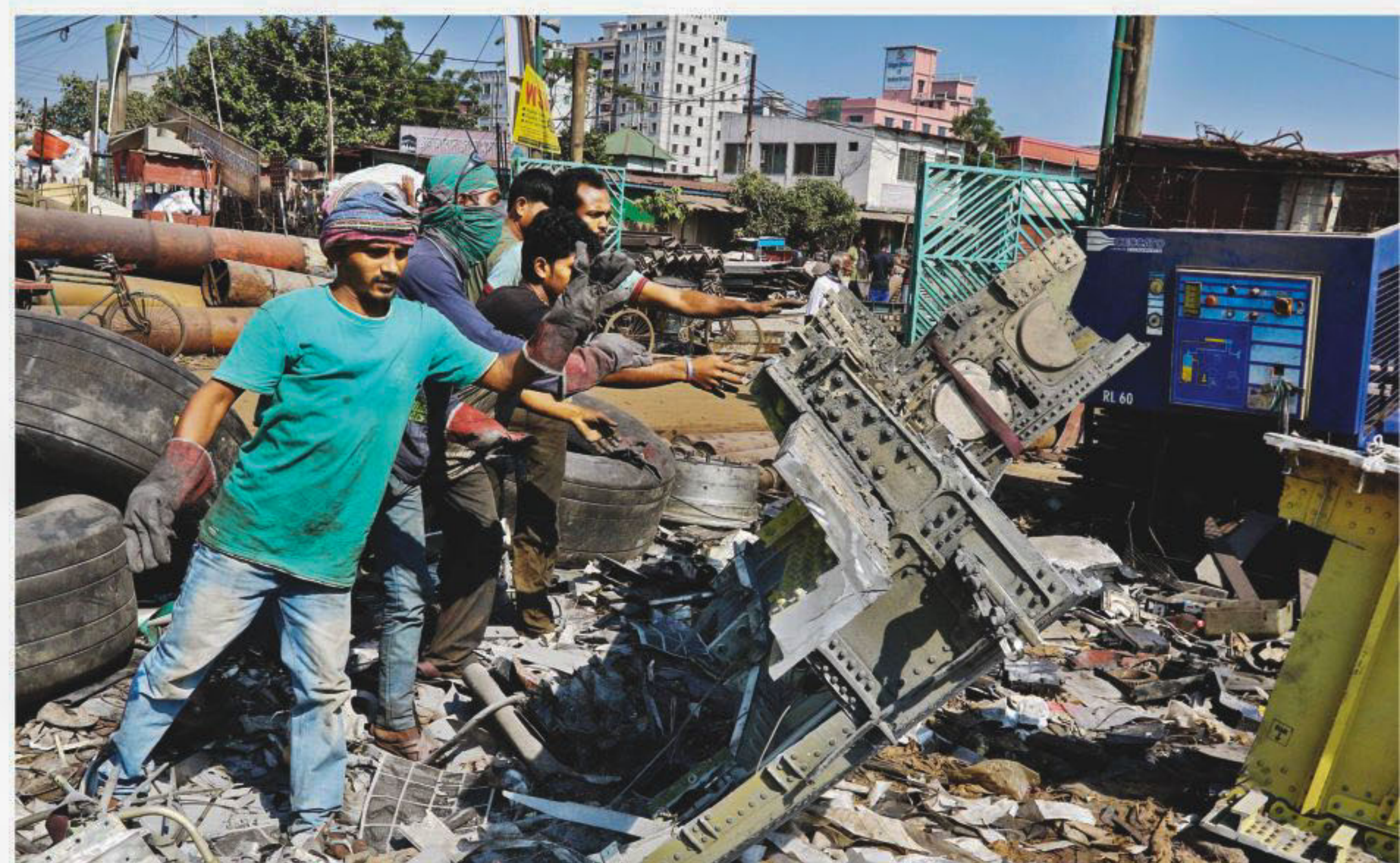
Tyres and disk brakes of a DC-10 are being taken away for melting and chunks of body is being cut into smaller bits to salvage the aviation-grade aluminium.
