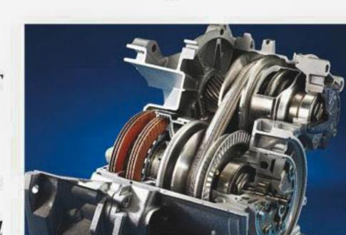
you B+ blood instead of A+. But generally, CVTs are quite sturdy and requires far less maintenance than the conventional automatics. The belt connecting the conical pulleys happens to be the most fragile unit of the CVT system and we spoke to the dealership service centers to find out ways of maintaining a CVT unit.
