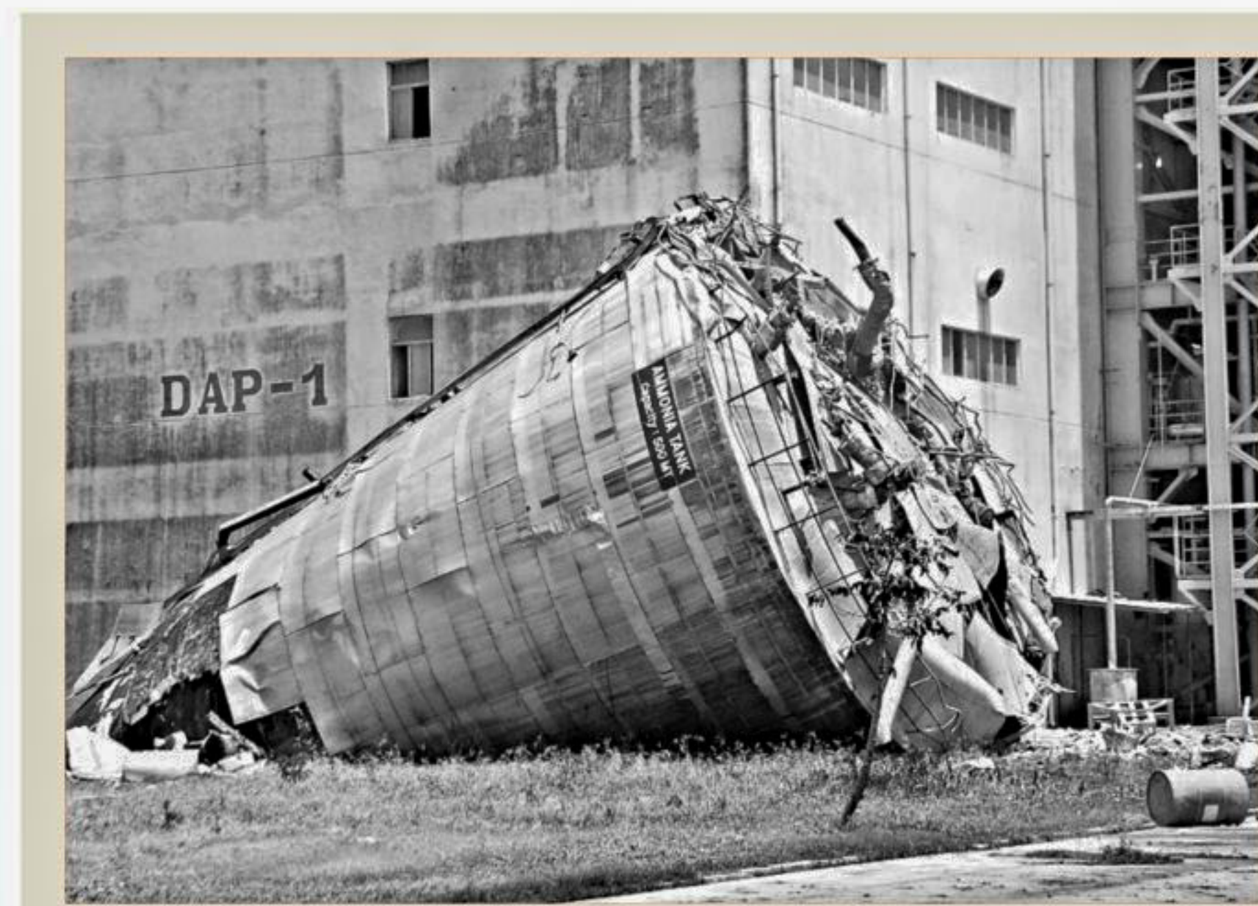
The damaged gas tank and pipes of DAP Fertiliser Company Limited in Anwara upazilla of Chittagong. An explosion at the factory caused the damage.
