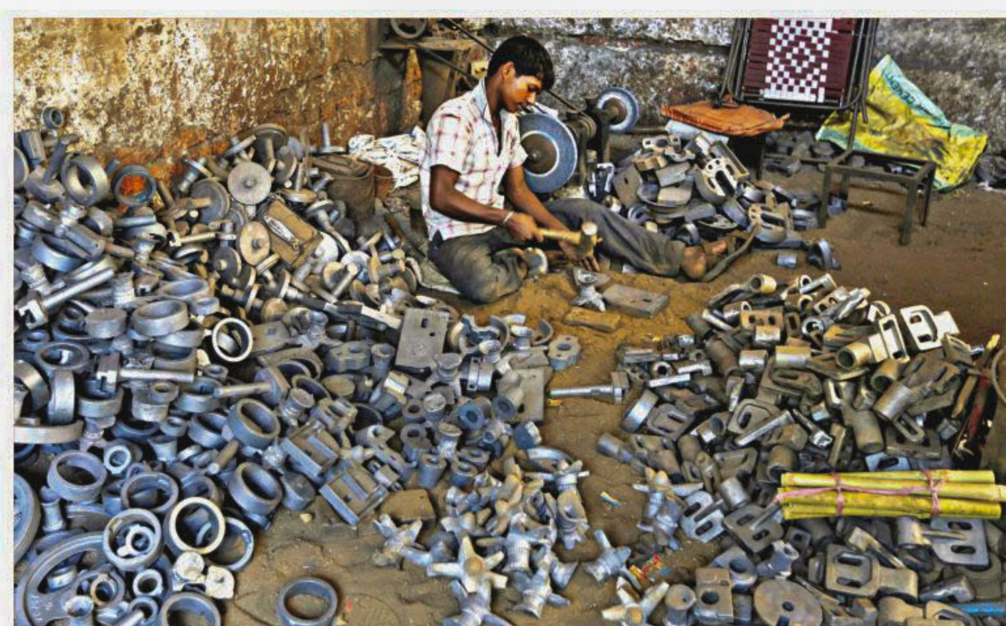
A worker separates casting joints of gearboxes inside a small-scale automobile manufacturing unit in Ahmedabad, India.
