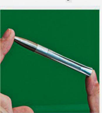
PROJECT EXACTO The EXACTO project is conducted by DARPA. It is a .50 caliber sniper rifle which has an onboard computer which allows it to change the bullet's direction 50 times per second using flaps. EXACTO can be used to precisely take down moving targets.
