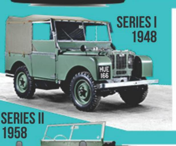
The original Series 1 came with just a 50 bhp 1.6 litre engine, and was meant for light industrial use. Inspired by the Jeep Willys, the Land Rover was exceedingly simple to operate, and use of steel and aluminium with solid build quality meant it lasted forever. LR estimates around 70% of them are still running like new.
