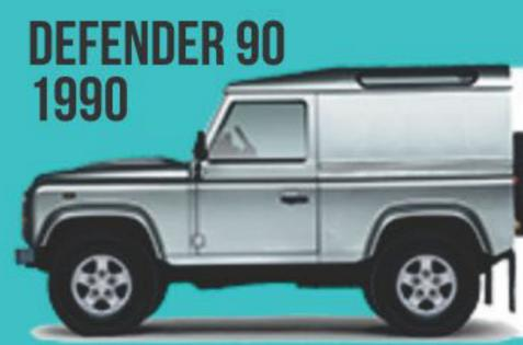
First one called "Defender" due to the introduction of the Discovery. It got modern suspension and a jump in the amenities, like air-con. The 90 name refers the short wheelbase.
