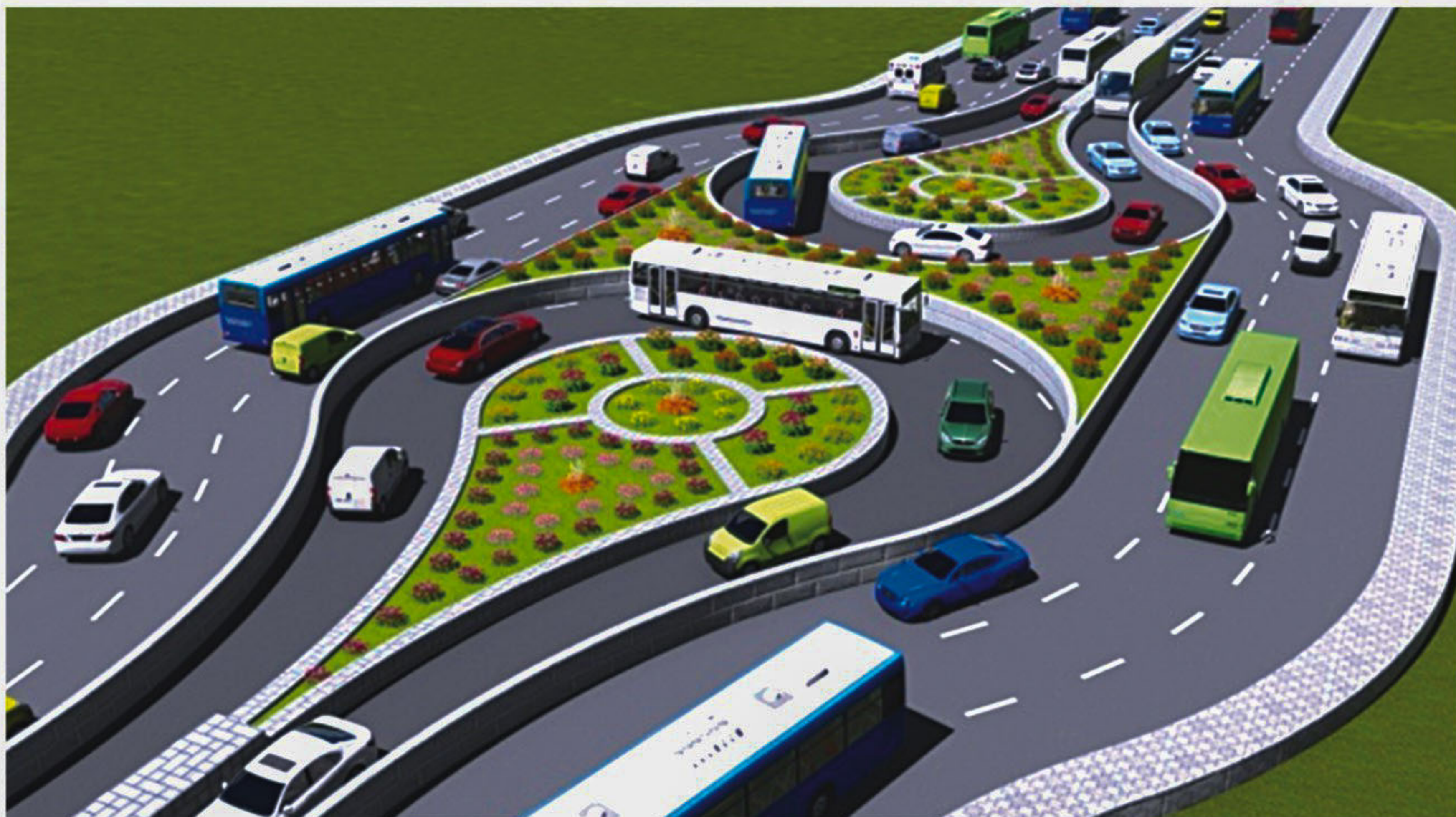
Type A U- loop, a CAD Image for buses and cars turnings
