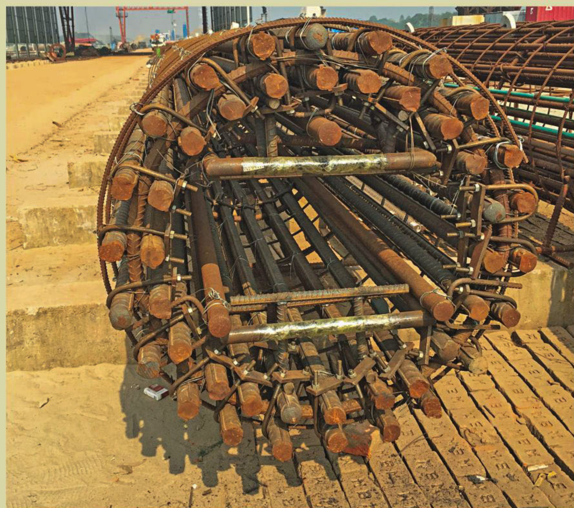
BSRM is producing 50 mm diameter reinforcing steel for the first time in the sub-continent.
