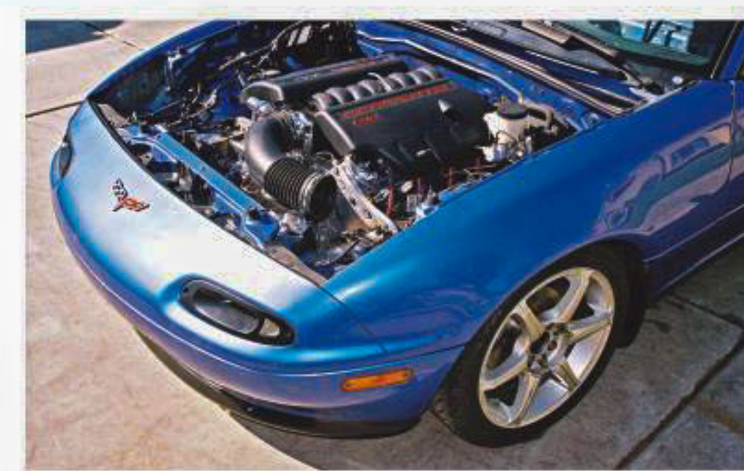
Chevy V8 in Mazda Miata. Tiny car, huge engine.
