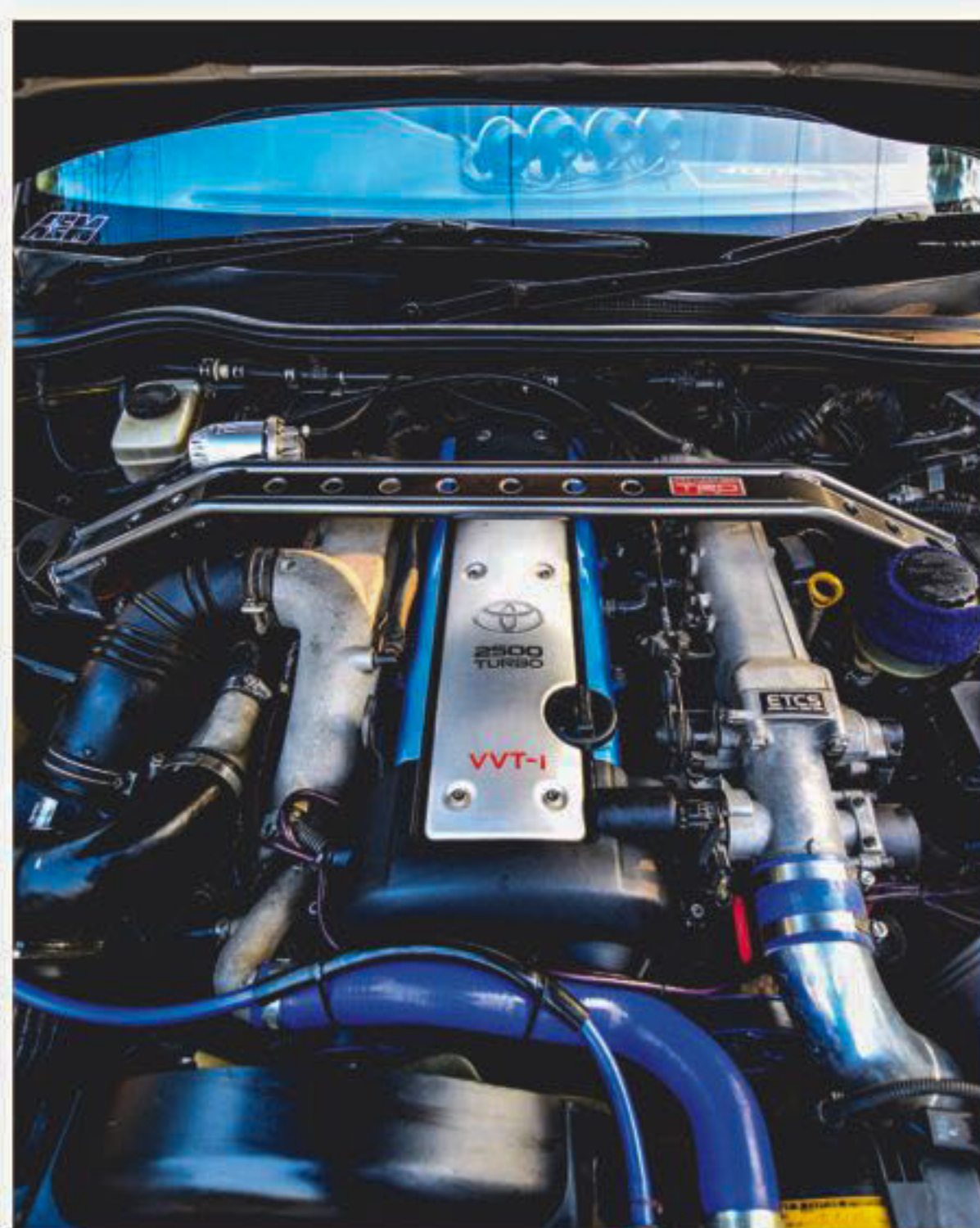
The 1JZ-GTE beast within Tanweer's Chaser. Some dream of Ferraris, others dream of 1JZ's.
