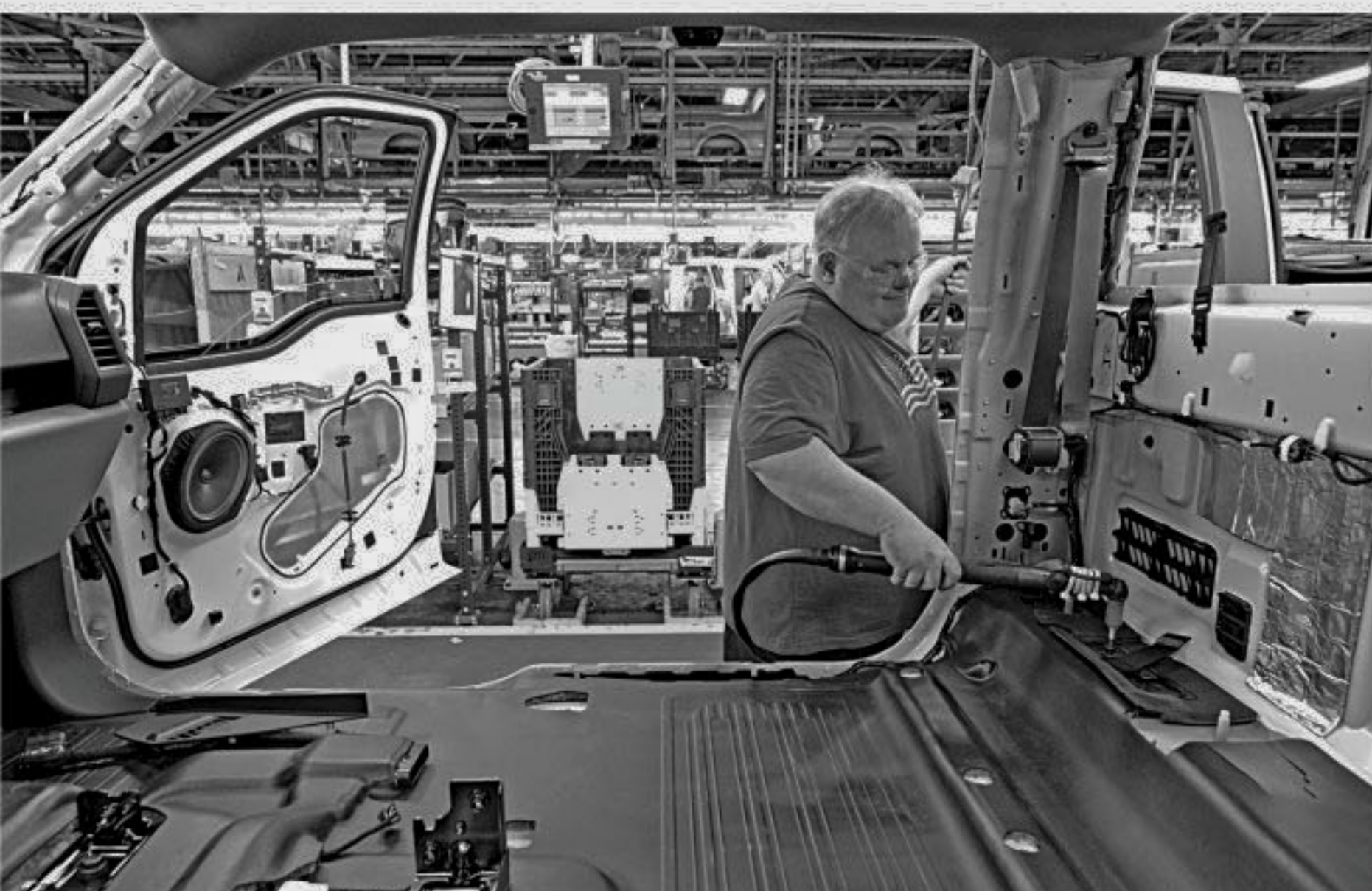
An auto worker screws a component into a cab in Missouri, the USA.
