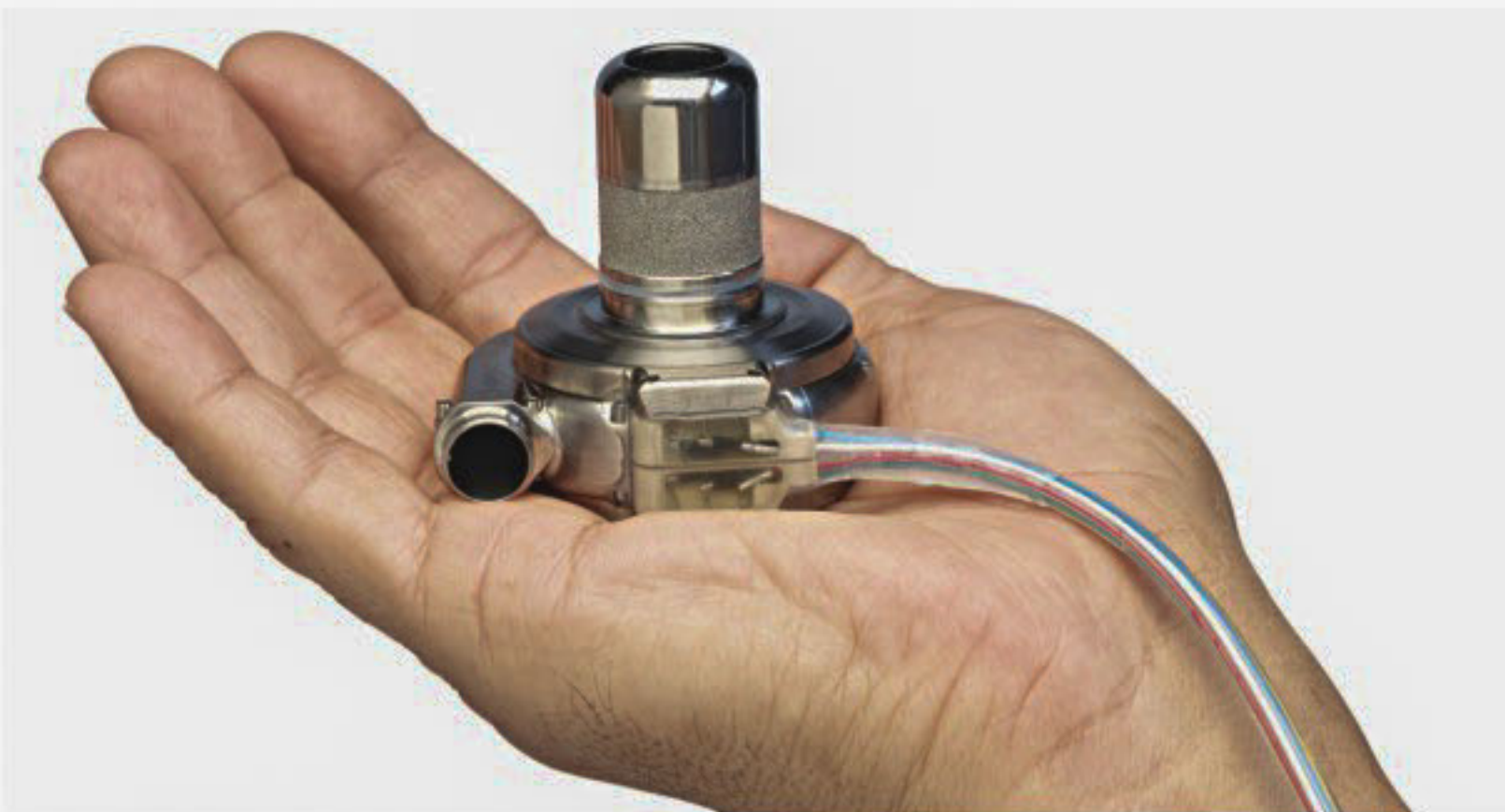
A HeartWare Ventricular Assist Device (HVAD) is held on a palm that works in association of some other parts including battery. The device is inserted by a minimally invasive surgery with the assistance of heart-lung machine.
