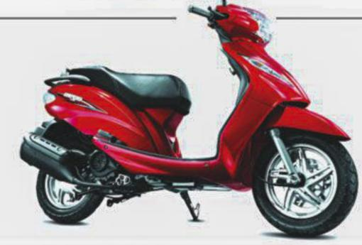
TVS Wego Price: 1,49,900 taka Displacement: 109.7 cc Max power/torque: 8hp@7500rpm, 8Nm@5500rpm Top speed: ~ 77 km/h Fuel consumption: 55 km/l Fuel tank capacity: 5 liters
