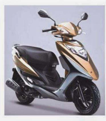
**Haojue Lindy** Price: TBD (To be determined) Displacement: 124 cc Max power/torque: 6.2 kW@7000rpm, 9Nm@6000rpm Top speed: ~ 75 km/h Fuel consumption: 58 km/l Fuel tank capacity: 5.8 liters
