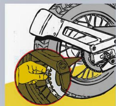
chain cover is that a rider wearing a sari or 'lungi' can get the garment tangled up. It also introduces the chain to dirt and water more easily. This accelerates wear and stretch.
