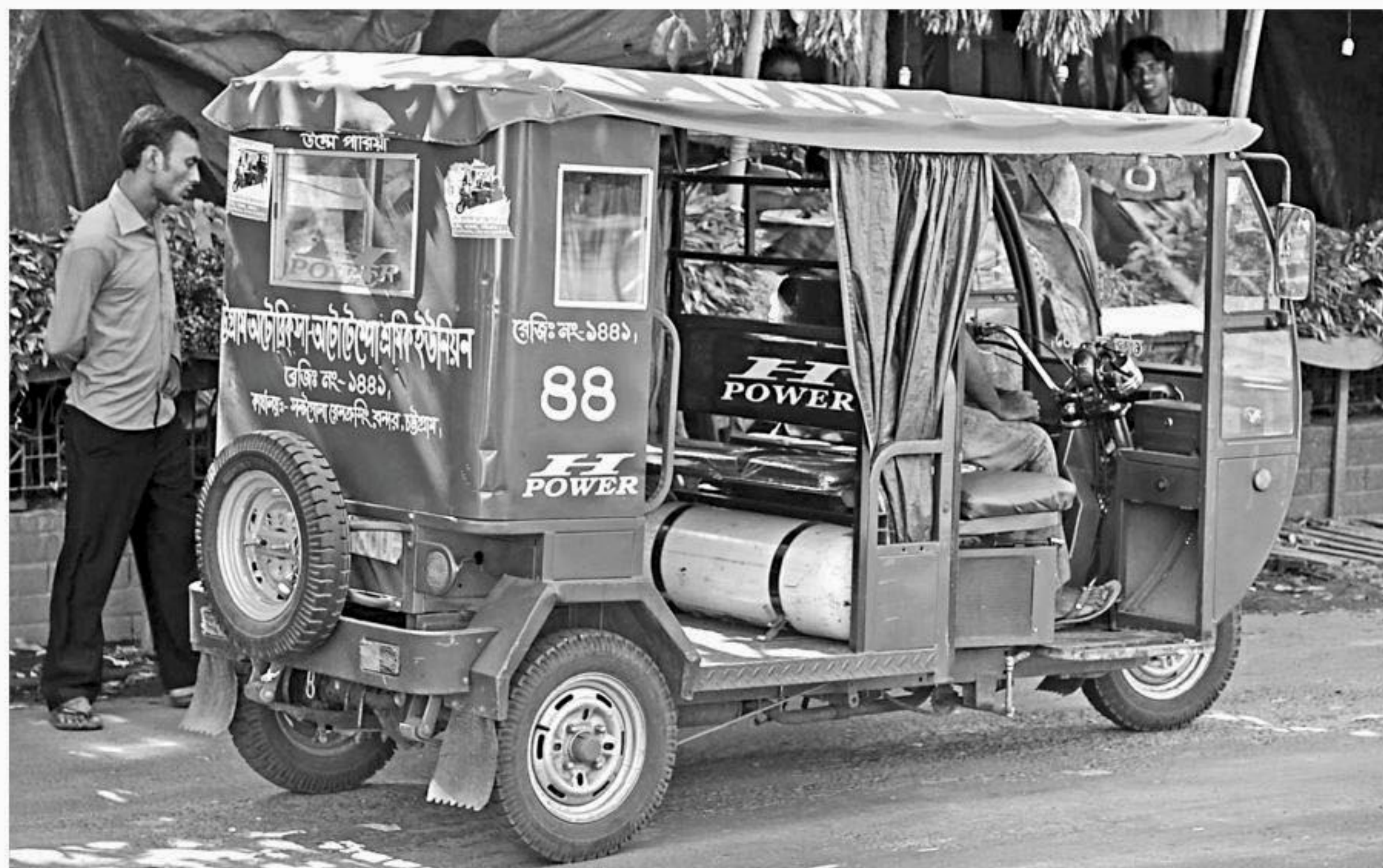
A recently imported CNG-run easy bike which has its gas cylinder right beneath the passenger seat, multiplying the risks of riding the shaky vehicle, in Chittagong city yesterday.
