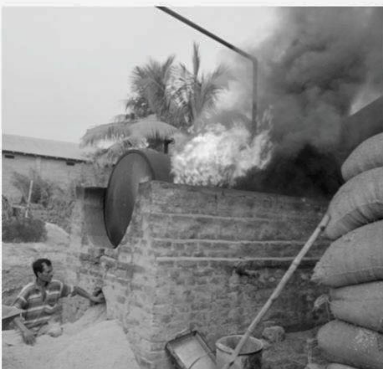
PHOTO: Exposure to Heat Radiation during manual husk feeding with traditional boiler system
