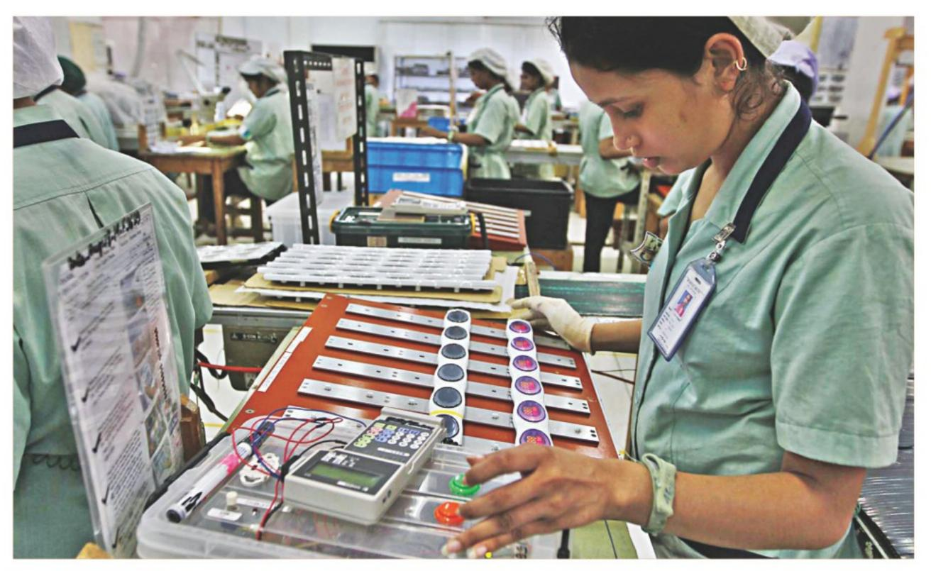
Bangladesh in Chittagong EPZ. The factory manufactures pushbuttons of vending machines widely used in Japan. It also supplies to the economic giant sophisticated devices like display boards at train stations, railway signals and LED lights.
