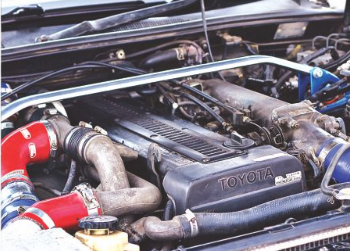
1JZGTE under the hood: Supra power for a Mark II.
